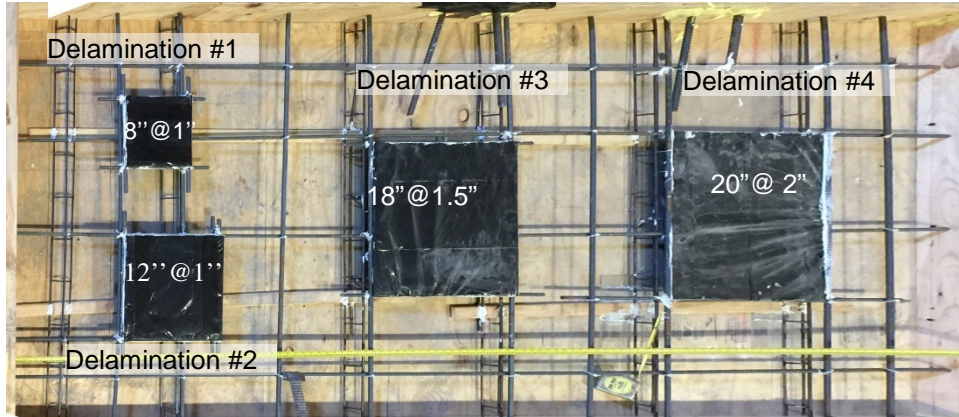
Figure 4-1 Concrete specimen with four artificial delaminations
