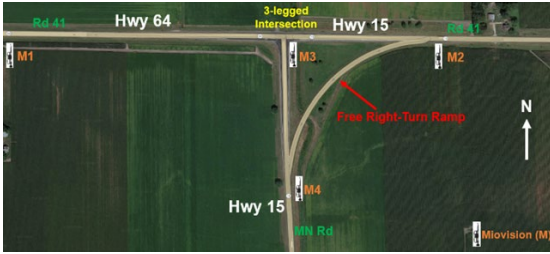
Site 1: Miovision installed in 3-legged FRT intersection
