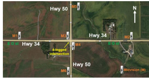
Site 4: Miovision installed in 4-legged non-FRT intersection
