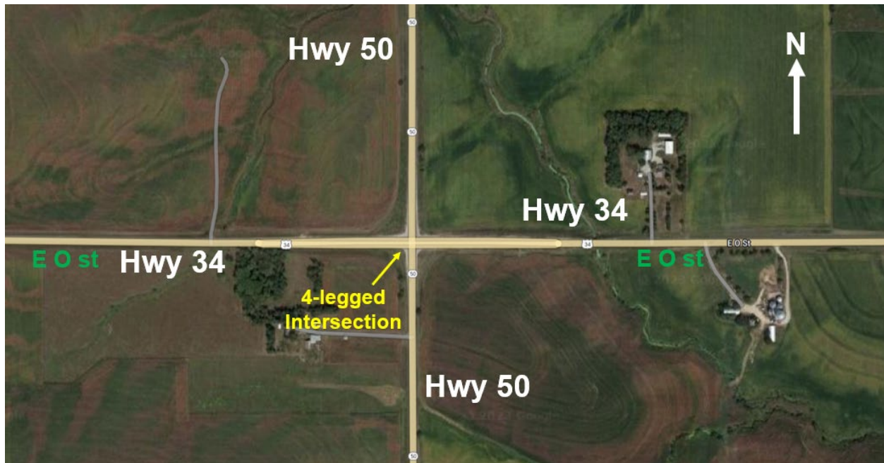
Figure 7.4 Four-legged Unsignalized Regular intersection at Avoca, Nebraska (Location coordinates: 40.813046, -96.178535)
