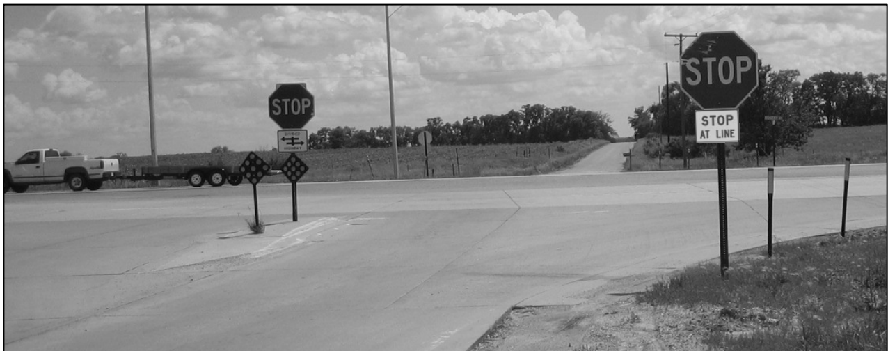
FIGURE 35 Example of Placement of STOP AT LINE Sign Only on Right STOP Sign on ORTL Project
