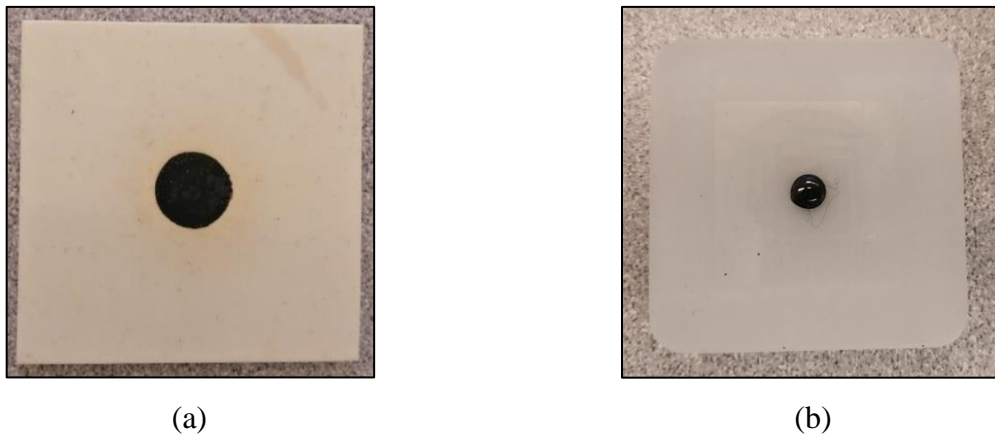
Figure 3.2 (a) 8-mm DSR mold (b) 4-mm DSR mold.
