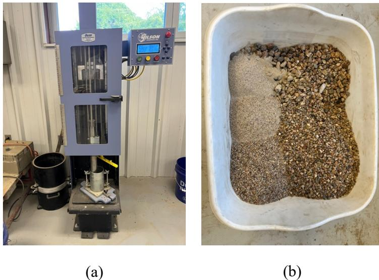
Figure 3.15 (a) Mechanical compactor (b) Sample material prepared following gradation
