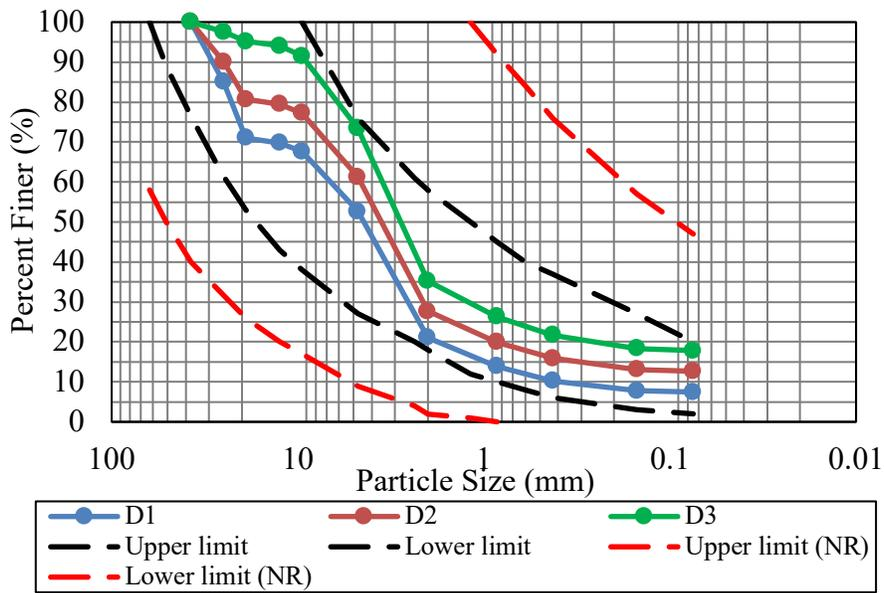
Figure 4.14 Gradation curves of the blends D1, D2, D3 with gradation recommended limits
