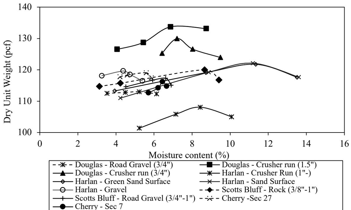
Figure 3.16 Proctor compaction curves for virgin surface materials
