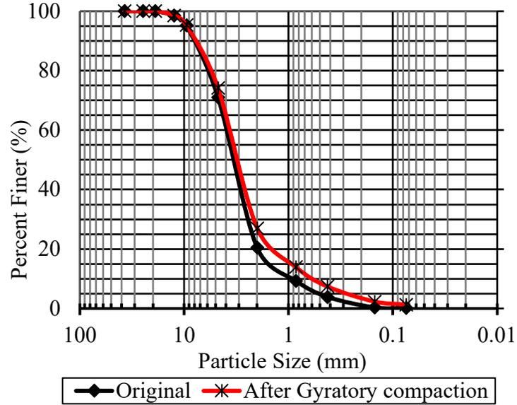
Figure A.2 Degradation of aggregates after gyratory compaction of DV3 (Road Gravel)
