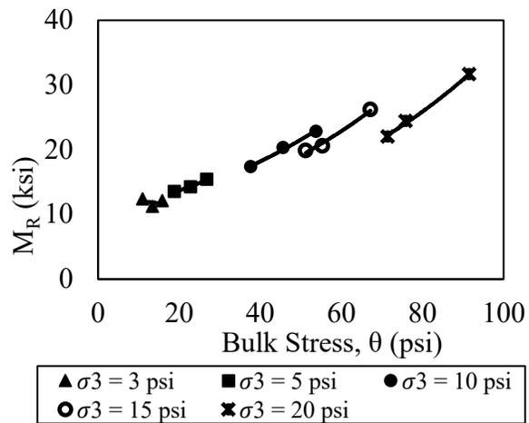
Figure B.34 Variation of Resilient Modulus with bulk Stress for Cherry blend C1 after 5FT
