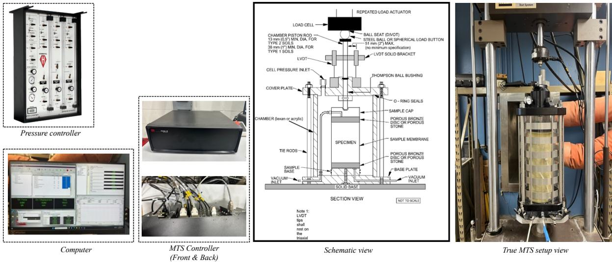
Figure 3.21 MTS 810 resilient modulus testing equipment setup
