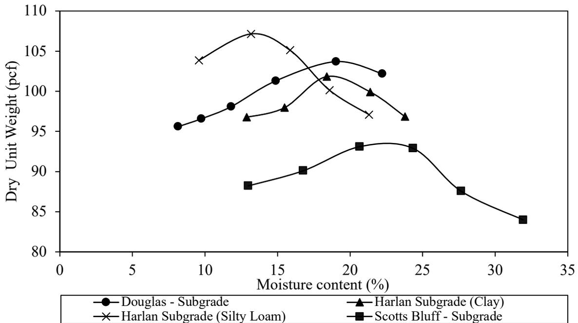
Figure 3.17 Proctor compaction curves for virgin subgrade materials
