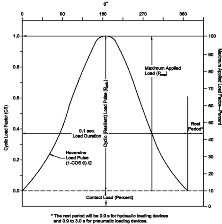
Figure 3.22 Cyclic axial load for Resilient modulus
