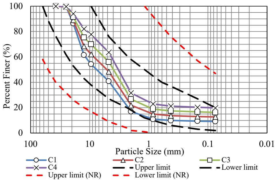
Figure B.14 Gradation curves of the blends C1, C2, C3, and C4 with recommended limits
