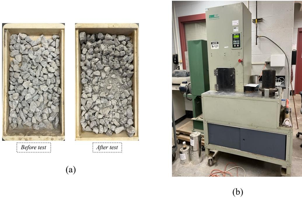
Figure 3.12 (a) Sample before and after test (b) Gyrotory compactor
