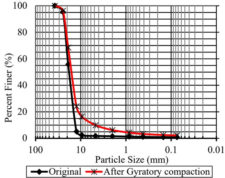
Figure A.1 Degradation of aggregates after gyratory compaction of DV2 (Clean 1.5'')
