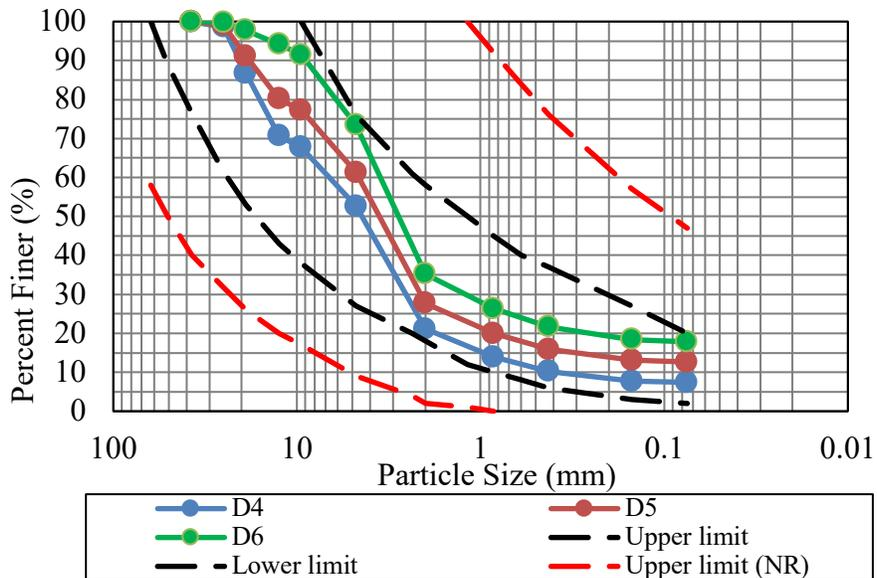
Figure 4.16 Gradation curves of the blends D4, D5, D6 with recommended limits
