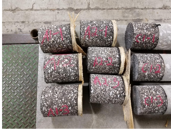
Figure 11. Density Test Cores for A Specimens
