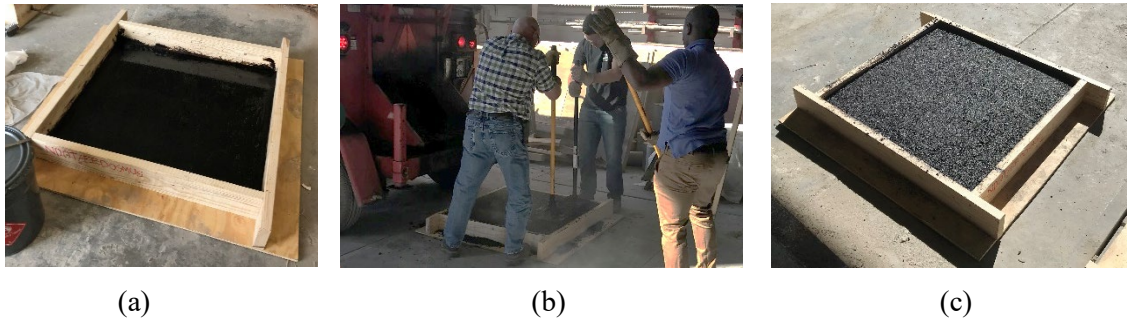
Figure 3. Specimen A1 (Asphalt only): (a) Primer Application, (b) Compaction, (c) Cast Specimen
