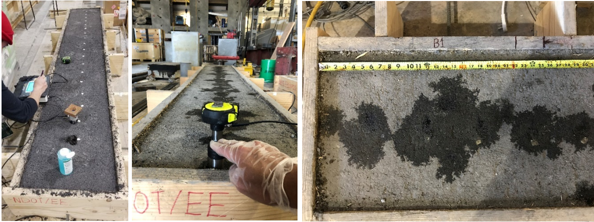
Figure 25. Segment by Segment Indirect UPV Testing of Specimen B
