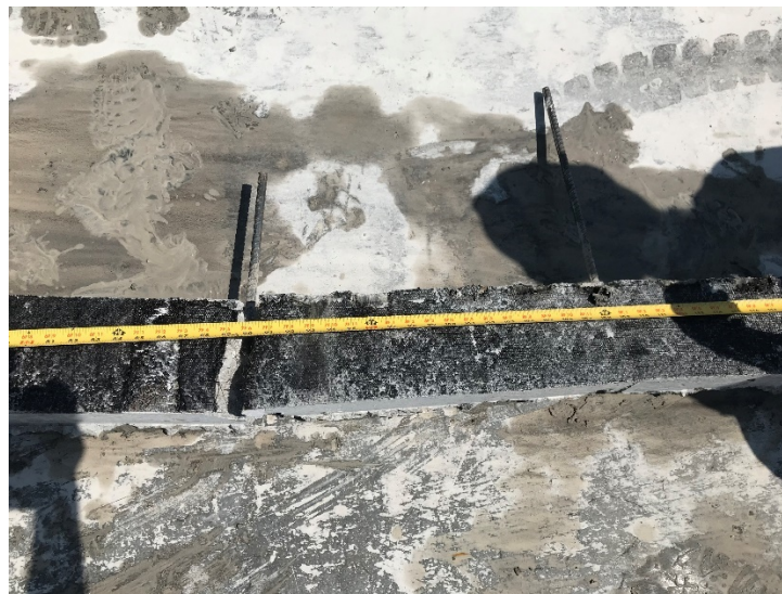
Figure 36. Segment B5: Status of Membrane After Testing
