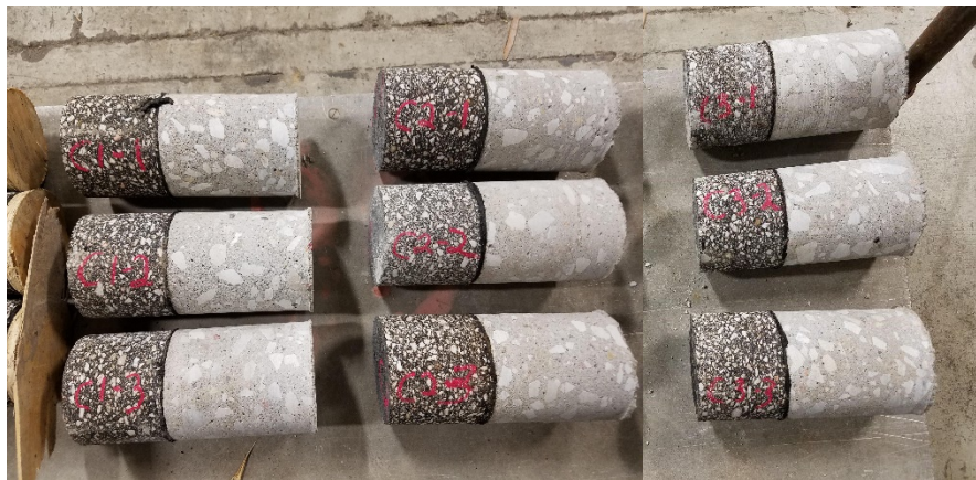
Figure 13. Density Test Cores for C Specimens
