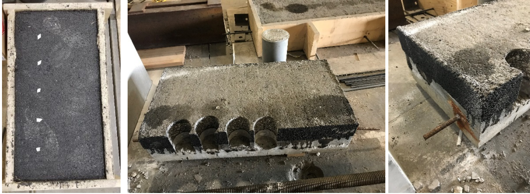
Figure 7. Images of Specimen C1: (a) After asphalt is cast, points show where receivers were placed in testing, (b) After the formwork is stripped and chloride testing is performed (cite paper), (c) Close-up of the corroded blunt-end (0-degree) rebar.
