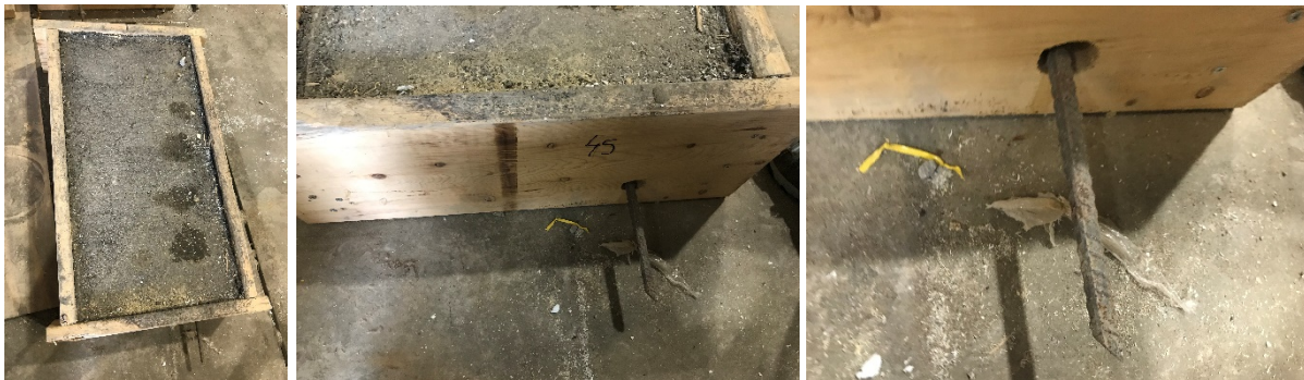
Figure 9. Images of Specimen C3 (45-degree end clan rebar)
