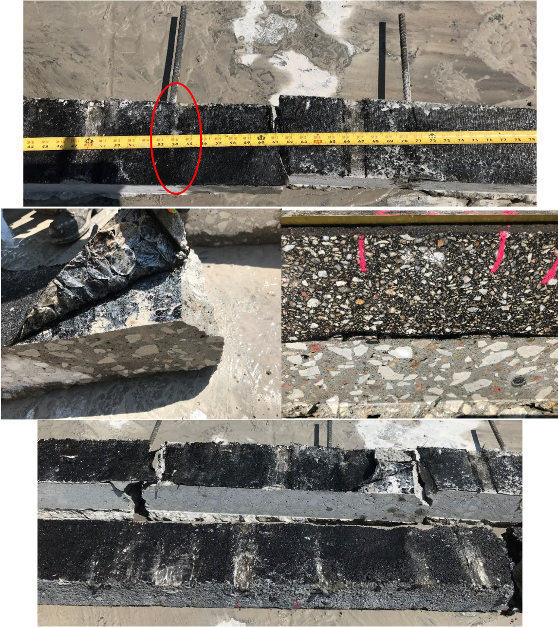
Figure 32. Segment B3: Status of Membrane After Testing
