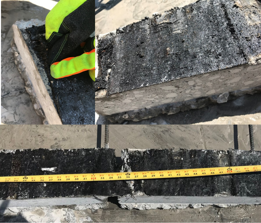
Figure 30. Segment B2: Status of Membrane After Testing
