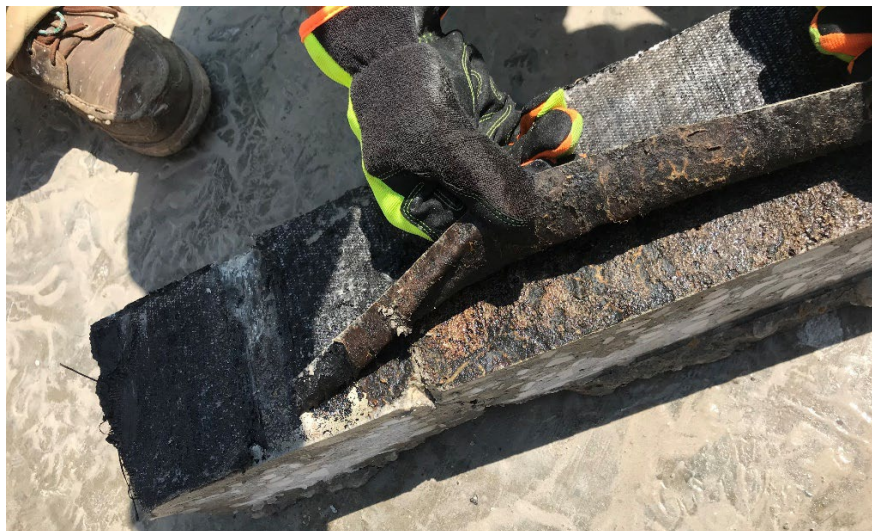
Figure 34. Segment B4: Status of Membrane After Testing
