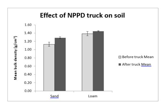
Fig. 5. The mean bulk density (g/cm³) of sand and sandy loam soil before and after a NPPD truck (30,000 kg) drove over it.
