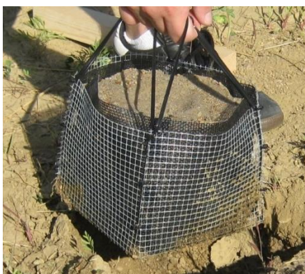
Figure 3.16 47-b media sediment collection basket deployed at I street
