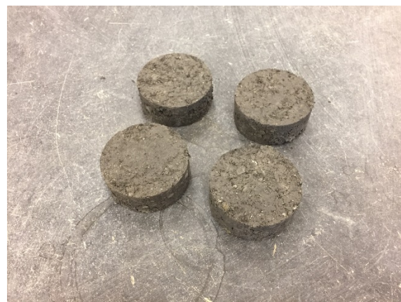
Figure D.5 Compacted samples after cutting and trimming
