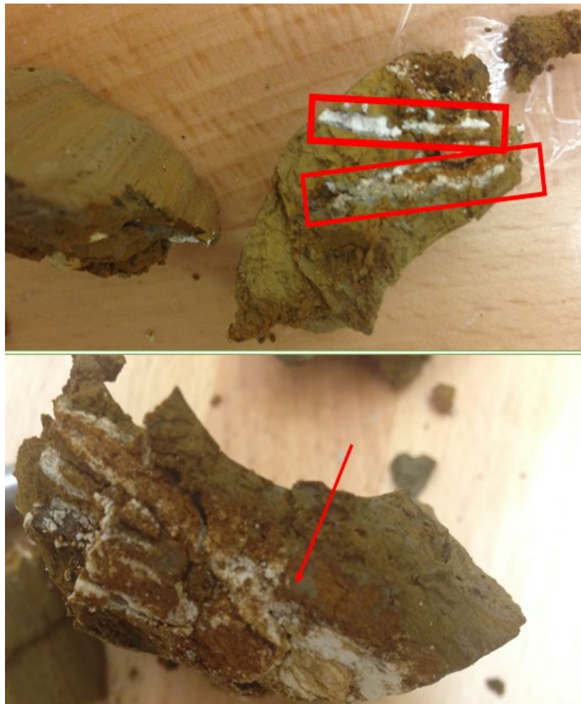
Figure 5.5 Layer of chawks (red arrow and boxes) in sample IS-19.5 (I-180 and Superior St.)
