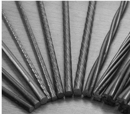
Figure E.10 Tendons for ground anchors: plain bars, threaded bars, strands from left to right
