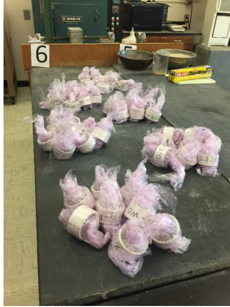
Figure D.6 Curing stabilized soil samples
