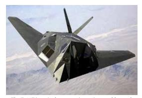
The F-117 is a single-seat, twin-engine stealth attack aircraft. Designed by Lockheed's "Skunk Works," the Nighthawk was not revealed to the public until 1988. (U.S.A.F. archival photograph)
