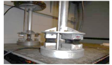
Figure 3. Concrete Blocks on Extension Machine
