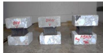
Figure 4. Concrete Blocks after 100% Extension — Visual Inspection
