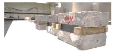
Figure 5. Concrete Blocks with Spacer Strips
