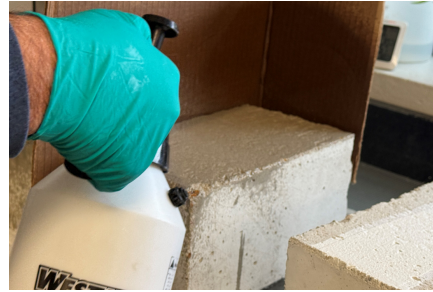
Figure 3: This image illustrates the application of sealer onto the slabs.
