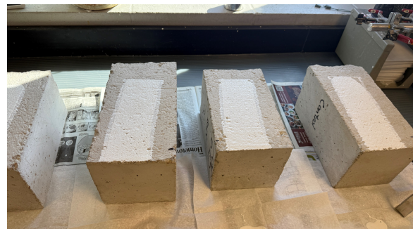
Figure 4: Concrete beams BHN-P, BHN-S, and Control are shown (from left to right) once all paint and sealer was applied.
