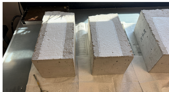
Figure 5: Concrete beams TK-P and TK-S are shown (from right to left) once all paint and sealer was applied.
