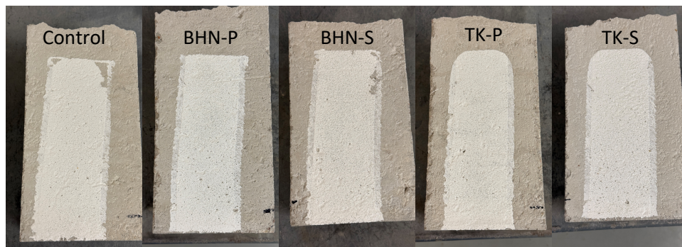
Figure 6: This image shows the 5 different concrete beams post scraping. While both Control and BHN-S had areas without paint, this was a paint application issue, not a paint adhesion issue. The paint was not applied at those locations.
