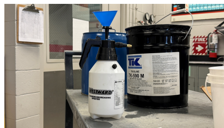
Figure 1: This image shows the two different sealers used, with TK-590 in the black and BHN in the blue. The white container is a standard sprayer used to spray sealer onto concrete beams in the lab.
