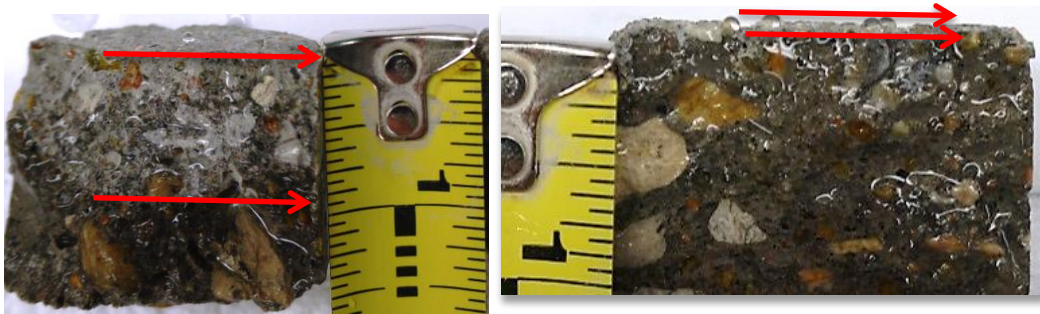
Figure 22 Contrast of a Good and Poor Depth of Penetration in a Split Core by the Visual Method
