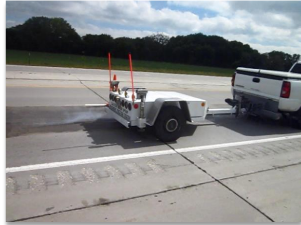
Figure 13 Determining of Skid Resistance with a Locked-Wheel Skid Tester
