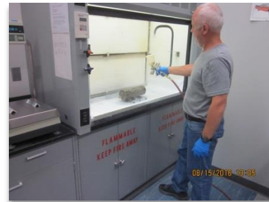
Figure 28 Sealer Application to Concrete Cores Using a Handheld Sprayer
