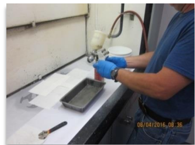
Figure 2 Handheld Sprayer for Sealer Application to Blocks
