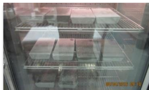
Figure 4 Hot Chamber for Laboratory Testing
