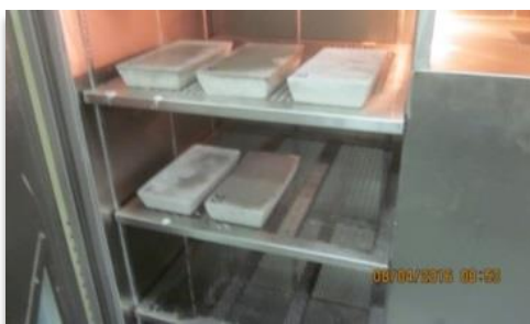
Figure 3 Cold Chamber for Laboratory Testing
