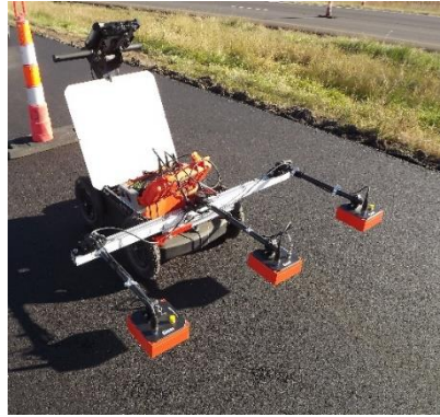
Figure 3. Rolling density meter (RDM) – Ground penetrating radar (GPR).
