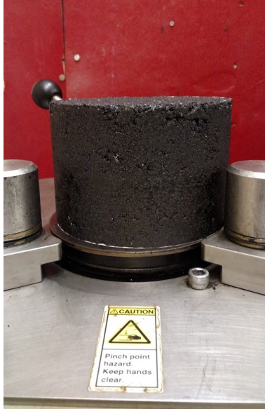
Figure 3-5. SGC compacted samples including interlayer.
