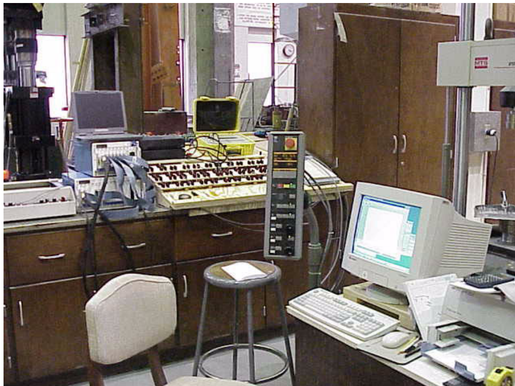
Figure 6-3: Data Acquisition and Load Control Systems
