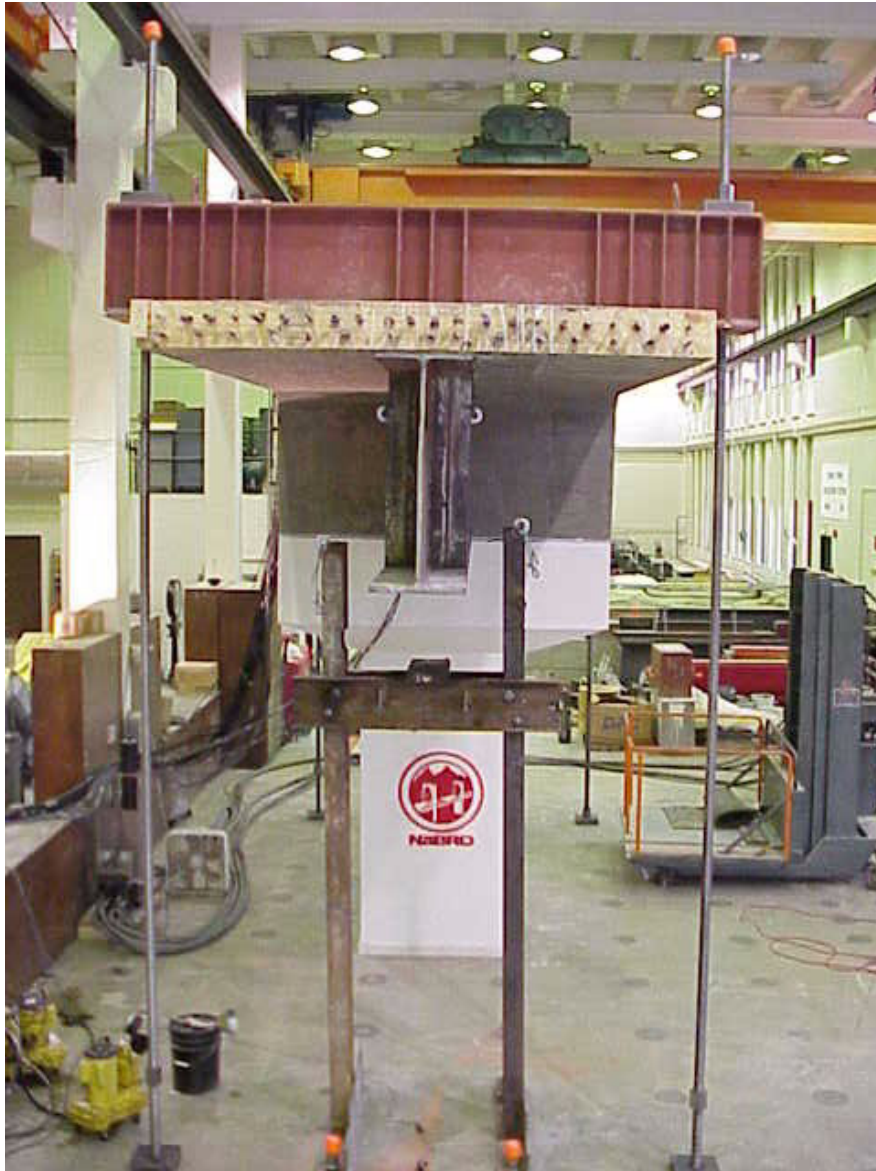
Figure 6-37: Ultimate Capacity Loading System (End View)
