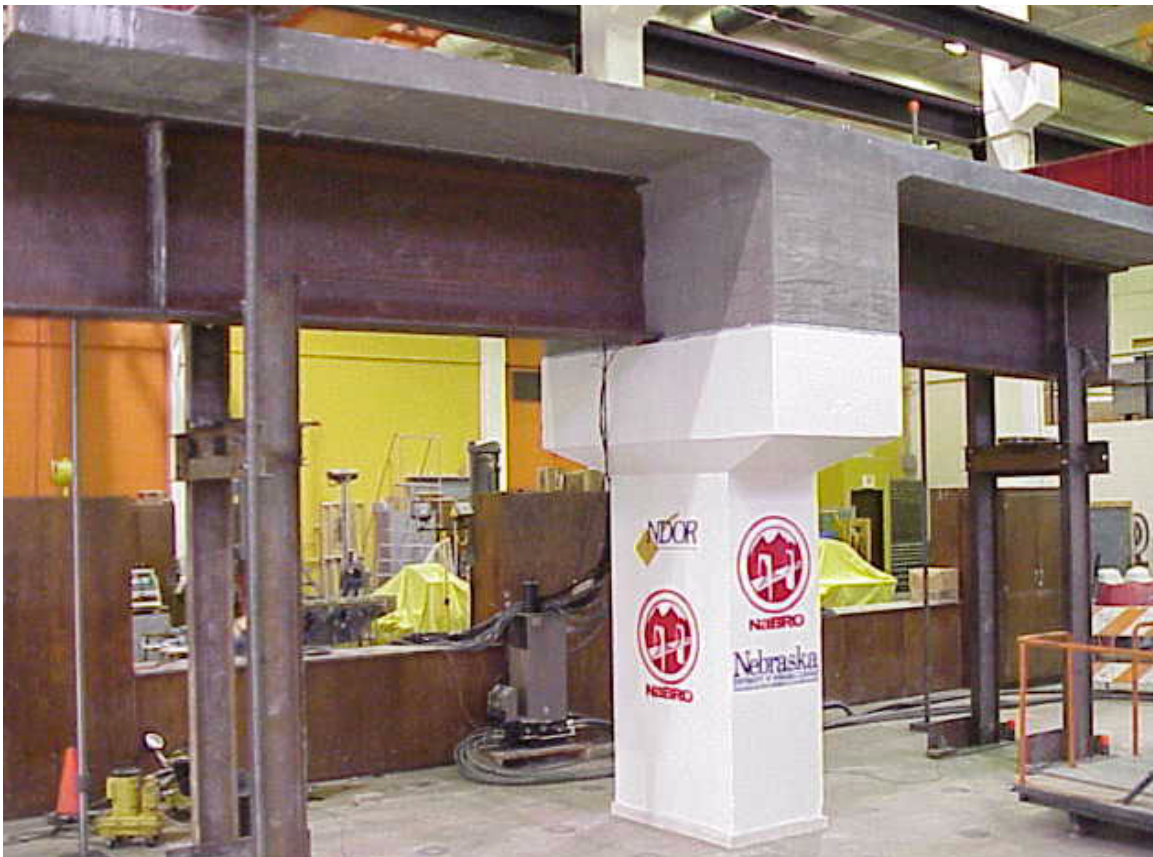
Figure 6-36: Ultimate Capacity Loading System (Side View)
