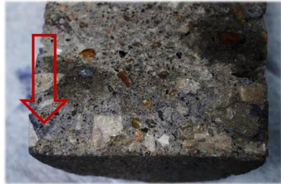
Figure 8 shows the Product 1 core. Slight blue dye can be seen on the sides of the core.
