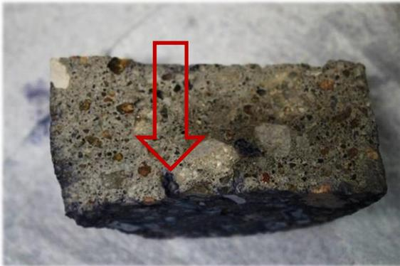
Figure 7 shows the control core. Slight blue dye can be seen penetrating at the surface.
