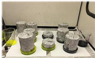
*Cores Submerged in dye solution*
