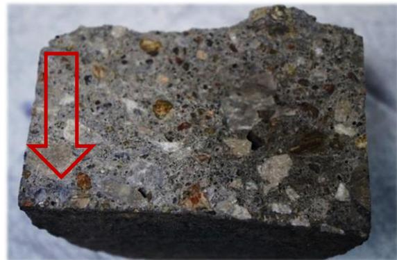
Figure 10 shows the Product 3 core. Slight blue shading can be seen in the left corner, caused by a chip in the surface.
