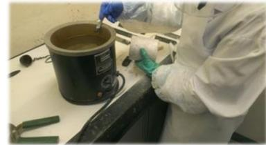
Figure 15 show the application of paraffin wax to the cores.
