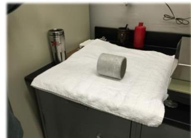
Figure 19 shows the surface drying of a previously submerged core before the measuring the final mass.
