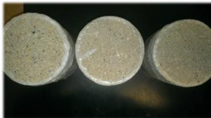
Figure 5 show cores sealed in wax.
