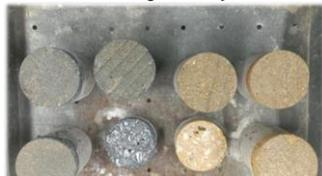
*Cores drying post submersion*
