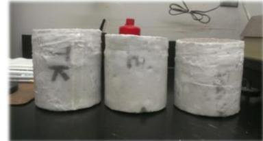
Figure 16 shows the cores with paraffin wax applied to the sides and bottom.
