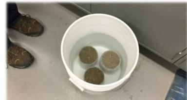
Figure 18 shows the cores submerged in water for 24 hours.
