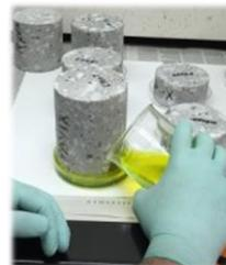
Figure 3 shows the yellow dye. Figure 4 shows submerged cores in yellow dye solution.
