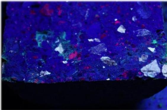
Figure 13 shows the Product 2 core with no coloring at the surface.
