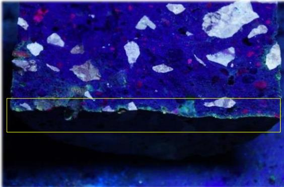
Figure 11 shows the control core with a very narrow band of coloring at the surface indicating no protection.
