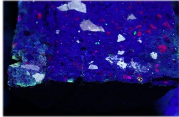
Figure 12 shows the Product 1 core with little to no dye observed at the surface. The left corner shows some fluorescence.
