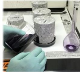
Figure 1 shows the blue dye. Figure 2 shows submerged cores in blue dye solution.
