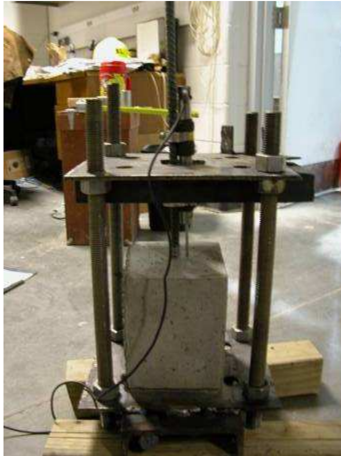
Figure 4.3.1 Pull-Out Test Setup – Method 1
