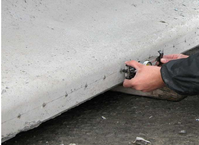
Figure 3.3.3 Transfer Length Measurement
