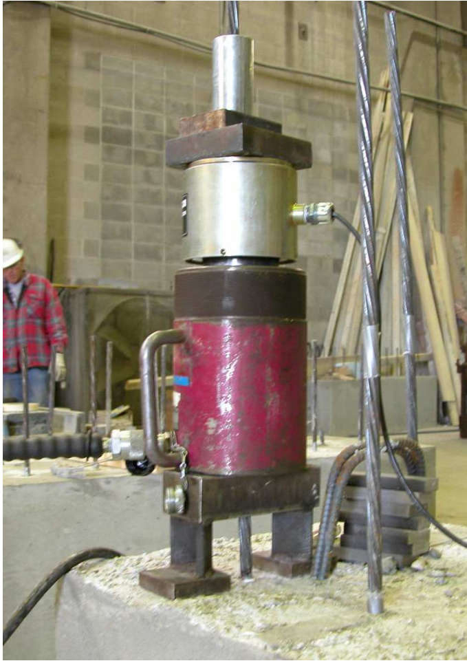
Figure 2.3.1 Moustafa Pull-out Test Setup
