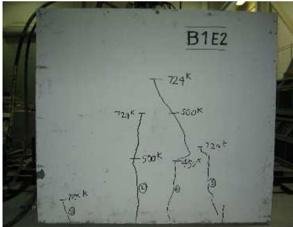
Figure 4.10 Crack of End Block at Failure of Specimen B1E2
