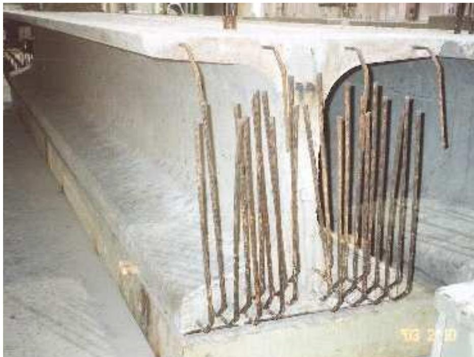
Figure 4.4 b) Bent Strands for Specimen B1E1
