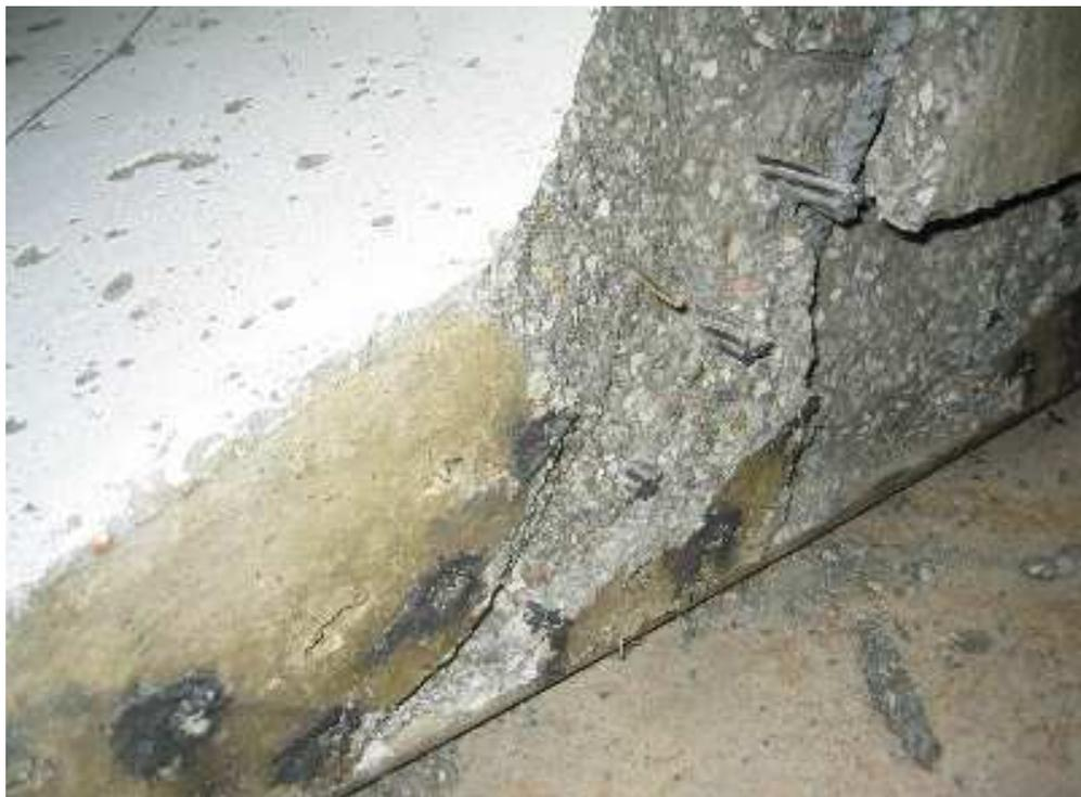
Figure 4.13 Shear/Bond Failure of Specimen B4E2
