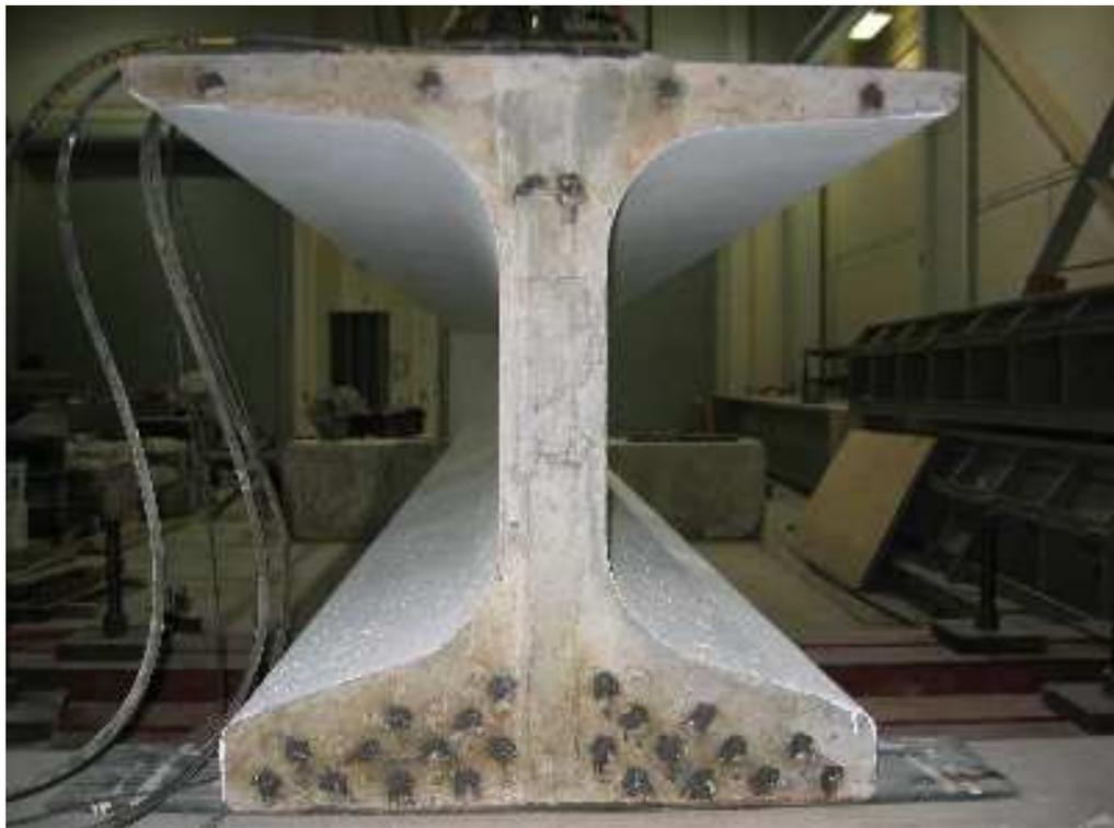
Figure 4.3 Beam End without End Block of Specimen B4E2
