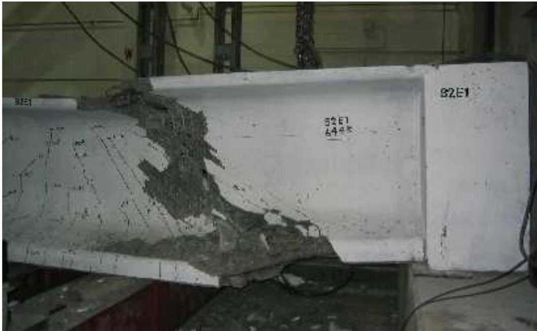
Figure 4.12 Pure Shear Failure of Specimen B2E1
