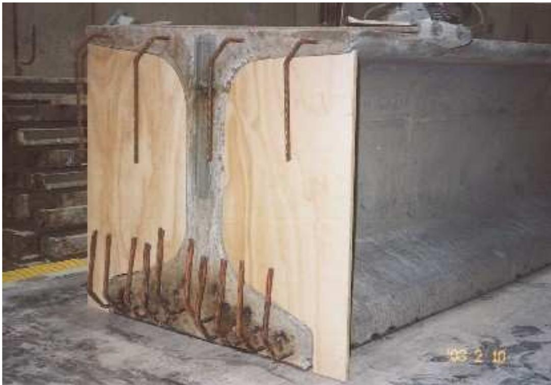
Figure 4.5 b) Bent Strands for Specimen B3E2
