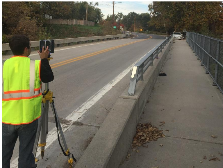
Figure 5.1: Deck scan setup for bridge S058 00994.
