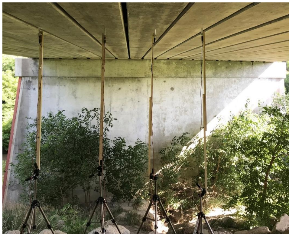
Figure F.9: LVDT setup for bridge S050 04149.
