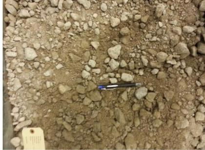
Figure 4 . Aggregate Sample for 40%RCA- 60% 47B Fine
