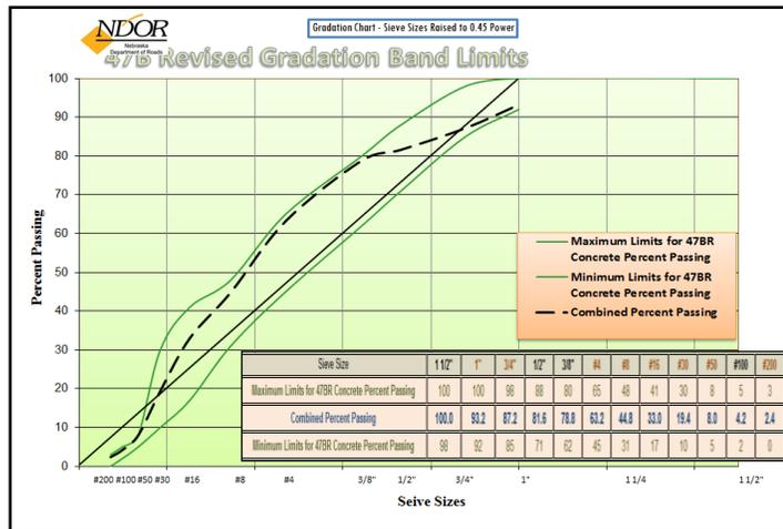
Figure 3. Combined Aggregate Gradations 50% RCA - 50% 47B Fine
