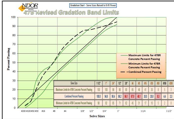
Figure 2. Combined Aggregate Gradations 40% RCA - 60% 47B Fine
