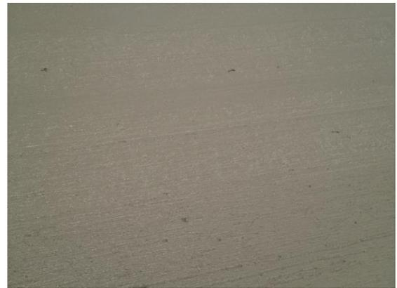
Figure 7. Placement Characteristic of 40%RCA-60% 47B Fine
