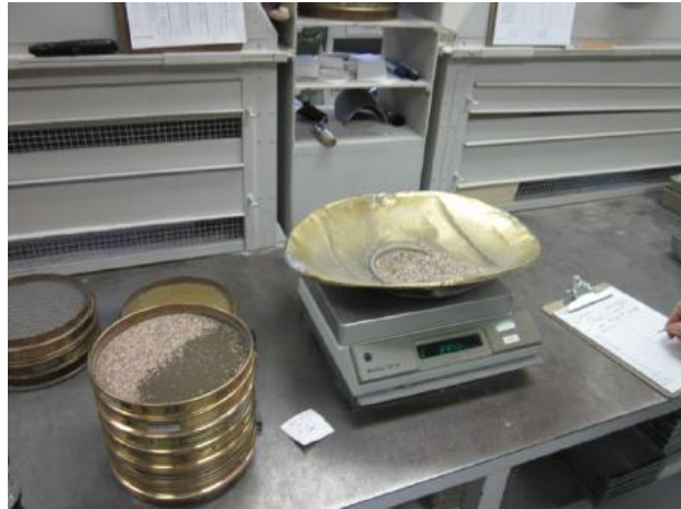
Figure 1. Weighing of Particles Retained on Each Sieve
