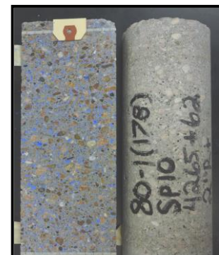
Figure 5. Core Visual Observation with Class B Fine Aggregate
