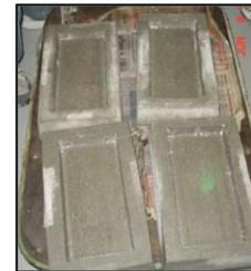
Figure1: Ponding block sets
