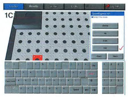
Figure 6.7: Selection of the measurement mode
