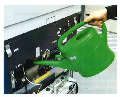
Figure 8.5: Refill of the deionized water reservoir
