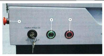
Figure 4.1: Control panel (including all switches)
