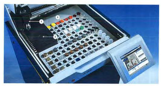
Figure 3.5: Inside the loader (sample magazine)
