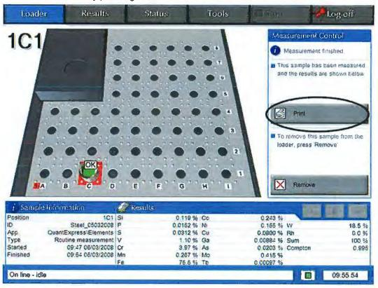
Figure 6.12: Results after the measurement
