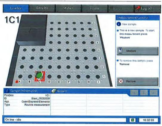
Figure 6.10: Start the measurement
