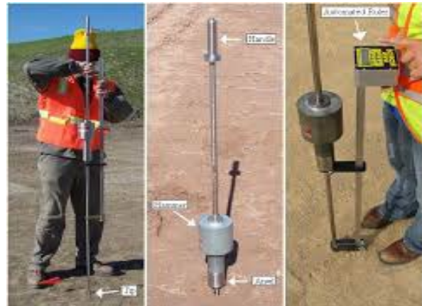
Figure 3 - Dynamic Cone Penetrometer (DCP) measures stiffness using inches per blow.
