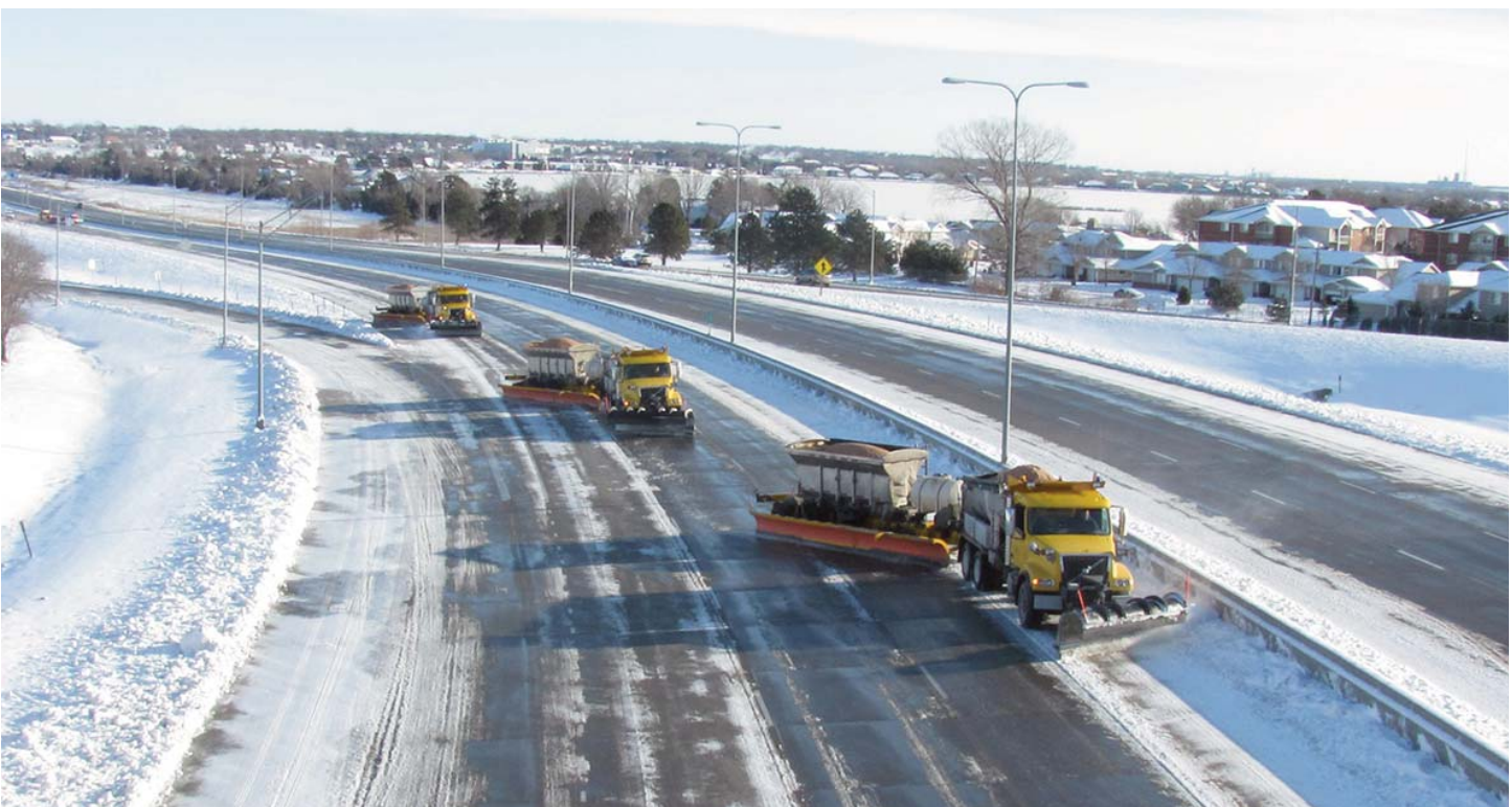
Three tow plows make their way along I-80, just east of the South US-77 interchange, headed west to Grand Island to help with snow removal operations.
