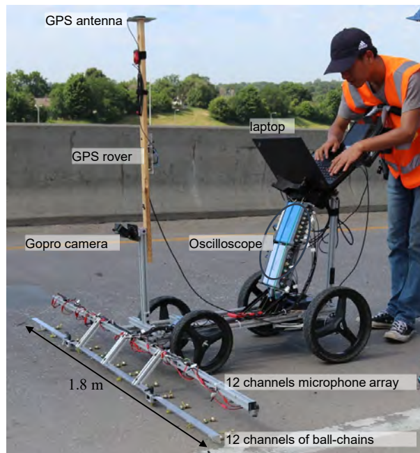
Fig. 3.4. 12-channel acoustic scanning cart
