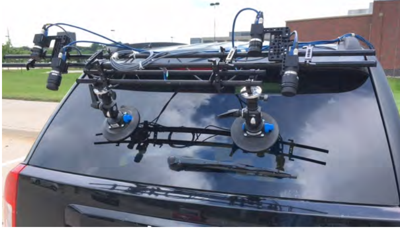
Fig. 4.3. Multi-view Camera System mounted on a Road Vehicle
