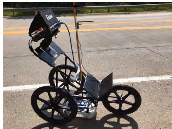
(b) GPR system on a survey cart
