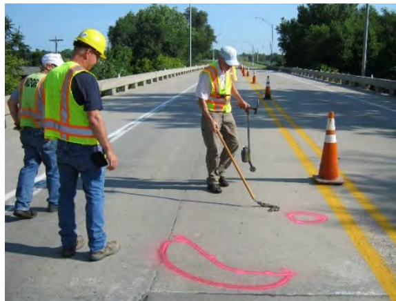
Fig. 1.1. State of the practice chain drag inspection on a bridge deck on which the locations of delaminations are marked using a handheld paint sprayer
