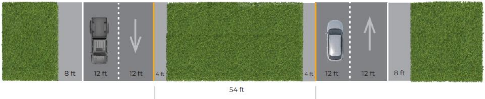
Existing Lanes (Resurfaced Pavement)
