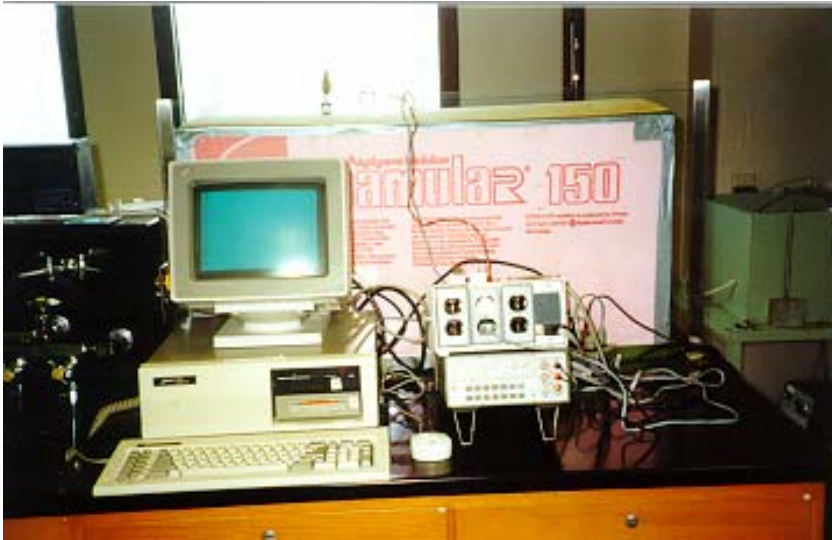
Figure 4-17 Temperature-controlled box for permeability test
