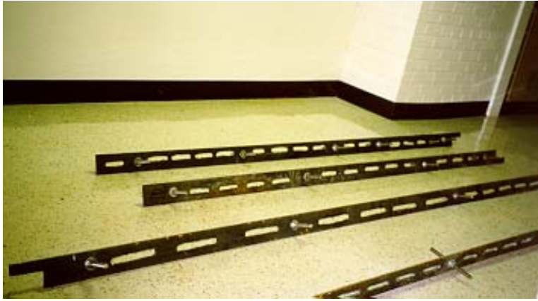
Figure 5-4 Steel plates with opening were used as electrodes
