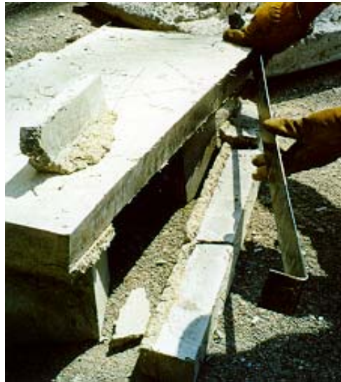
Figure 3-16 Smooth surface between the steel plate and concrete surface
