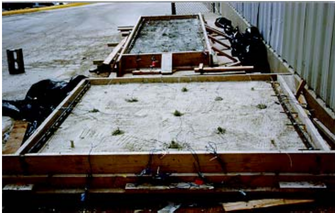
Figure 5-9(b) Thermocouple layout before casting overlay
