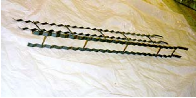
Figure 3-17(c) 3/4 in. corrugated steel plate welded on steel posts with 1.25 in. spacing
