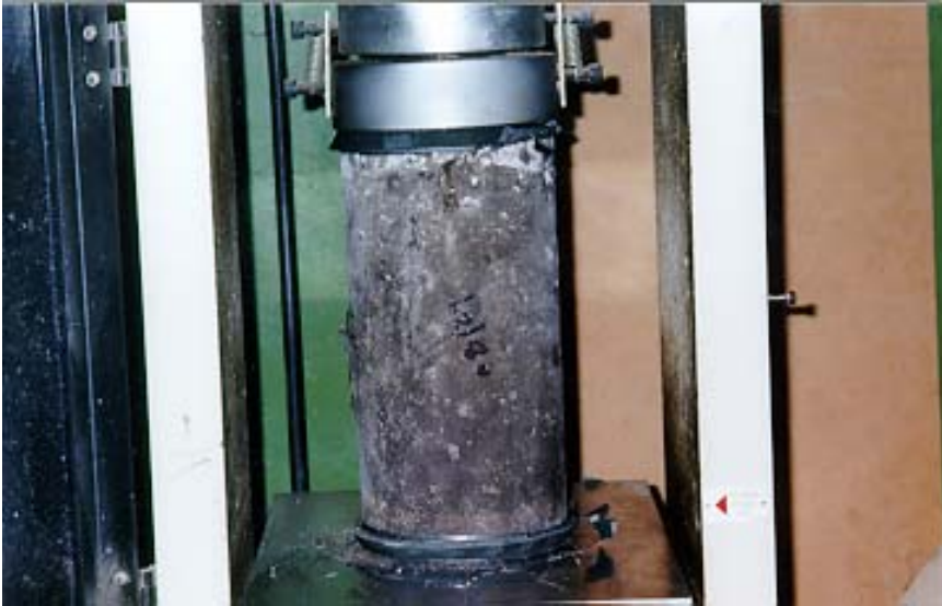
Figure 4-4 Typical failure mode of concrete in compression
