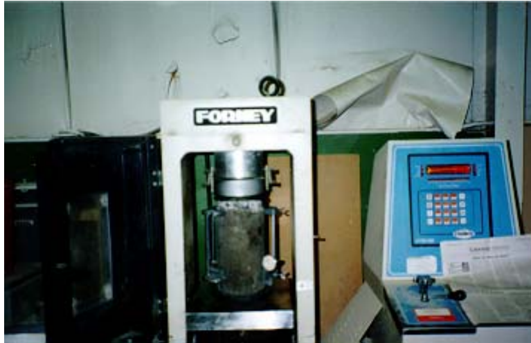
Figure 4-5 Test setup for stress-strain relationship
