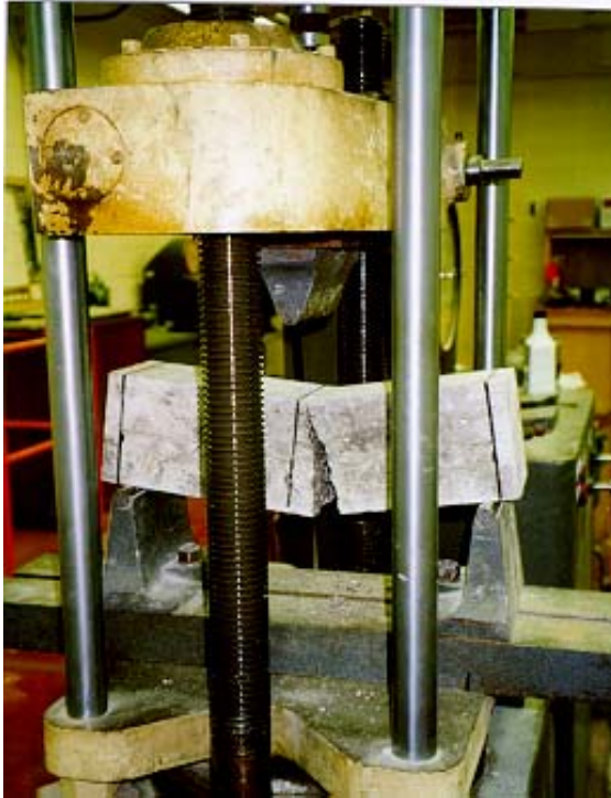
Figure 4-8 Flexural strength – test setup
