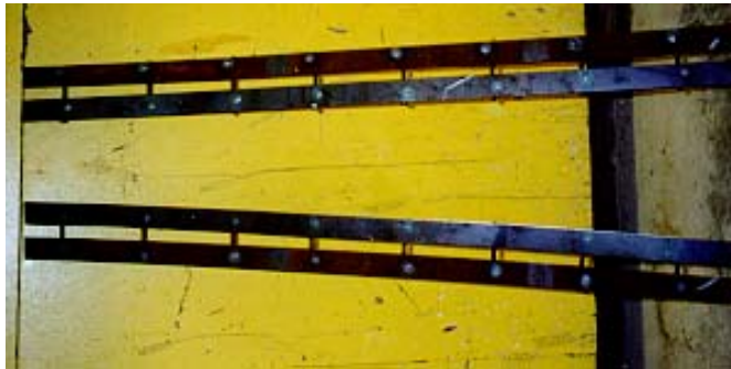
Figure 3-17(b) 1 in. steel plate welded on WWF with 0.5 in. spacing
