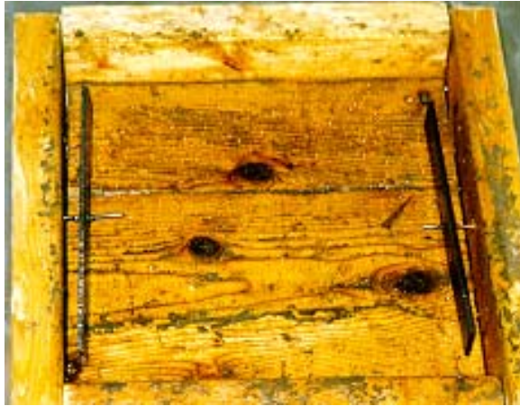
Figure 3-6 Steel plates are used for electrodes
