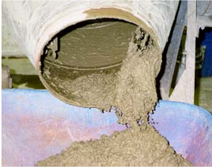
Figure 3-4 Typical conductive concrete mix
