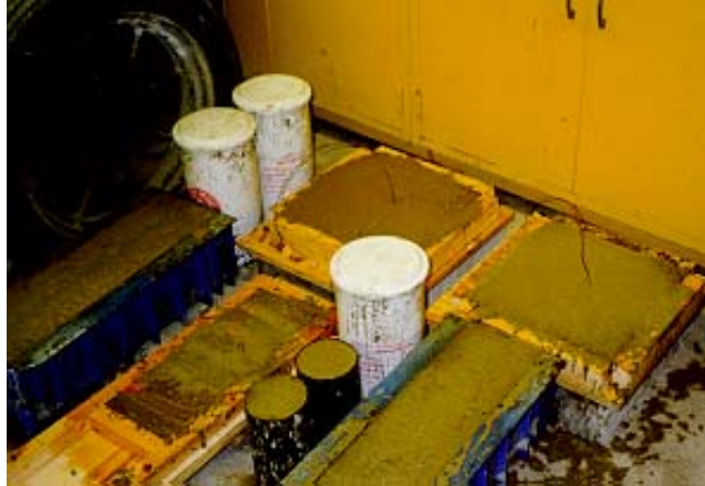
Figure 3-9 Conductive concrete test specimens Category 3 (stage two evaluation)
