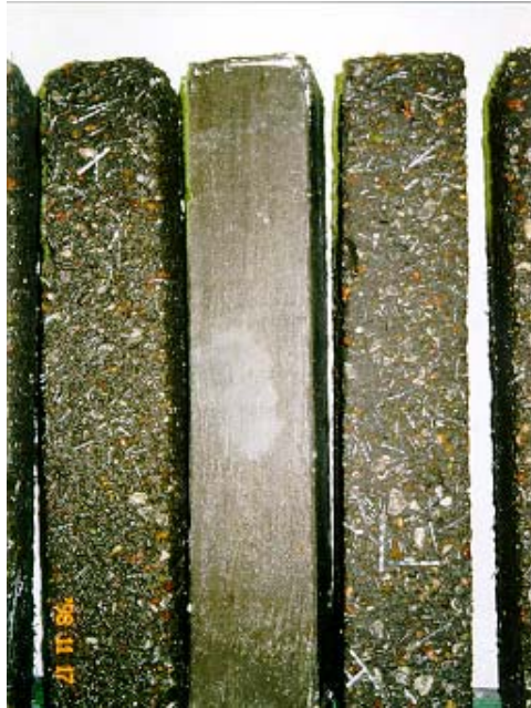
Figure 4-12 Freeze and thaw specimens – before and after 312 cycles
