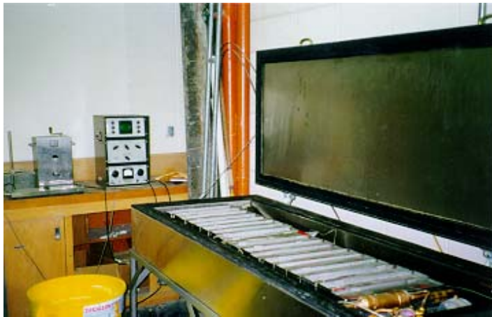
Figure 4-10 Freeze and thaw testing equipment
