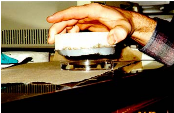
Figure 4-18 Permeability test specimen preparation
