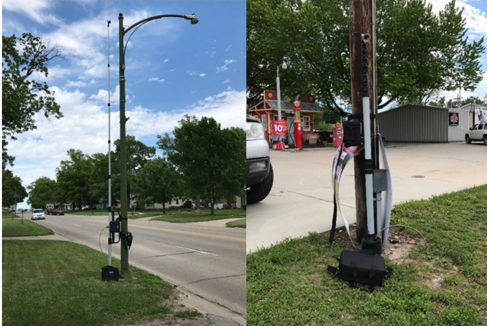
Figure 3.3 Setup of Miovision Scout cameras
