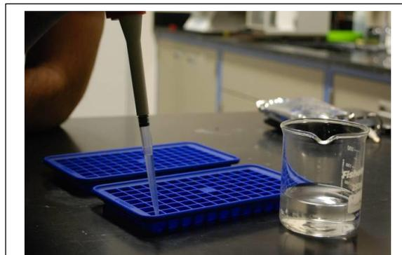
Figure 4 - Pipette 1.3 mL water into ice cube trays.
