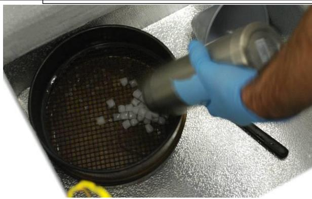
Figure 11 - Emptying the thermos contents into the sieve. (Tuan & Albers, 2014.)
