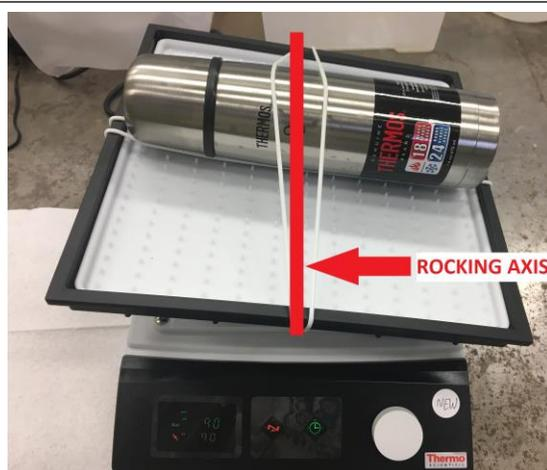
Figure 10 – The Thermos is oriented perpendicular to the rocking axis on the Thermo Scientific Rocker in the NDOT chemistry lab. (NDOT 2018).
