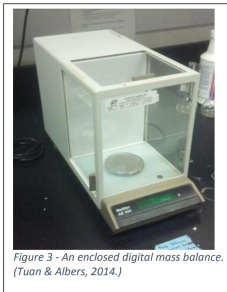
Figure 3 - An enclosed digital mass balance. (Tuan & Albers, 2014.)
