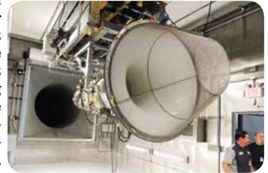
Falcon 900 Engine in Test Cell with Protective Engine Inlet Cover
