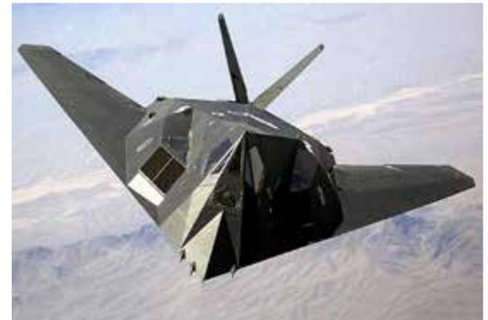
The F-117 is a single-seat, twin-engine stealth attack aircraft. Designed by Lockheed's "Skunk Works," the Nighthawk was not revealed to the public until 1988. (U.S.A.F. archival photograph)
