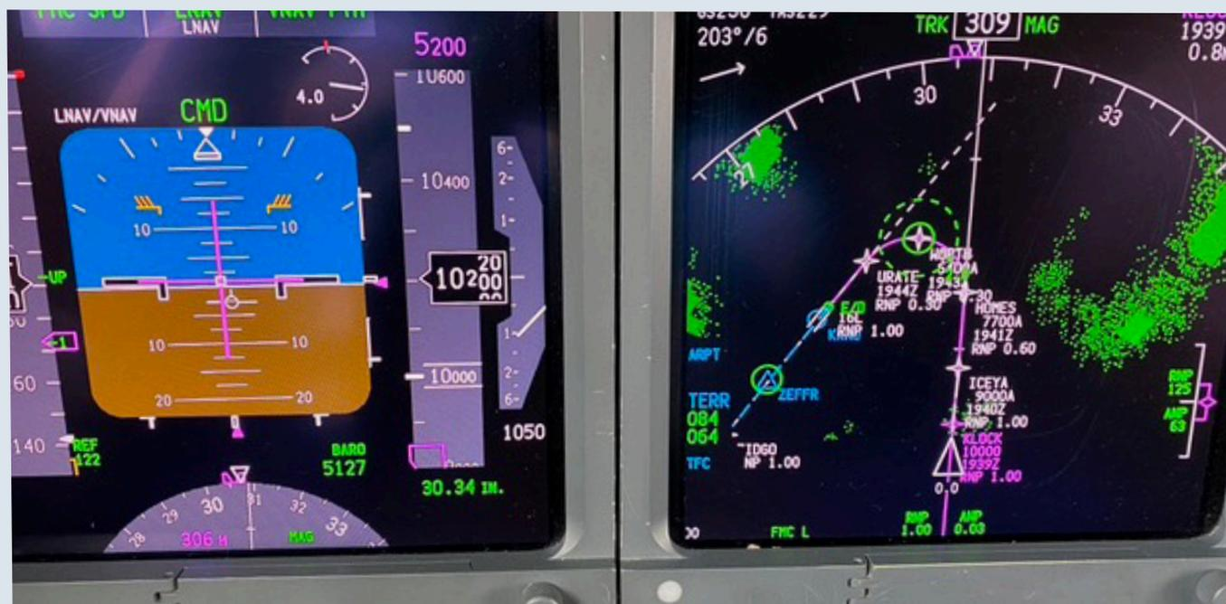
Onboard radar shows a Required Navigational Performance (RNP) approach to 16L into Reno. All needed information is on the Primary Flight Display as well as the Navigation Display. The whole route can be seen with fixes, altitudes, terrain, and all of the primary flight data.
