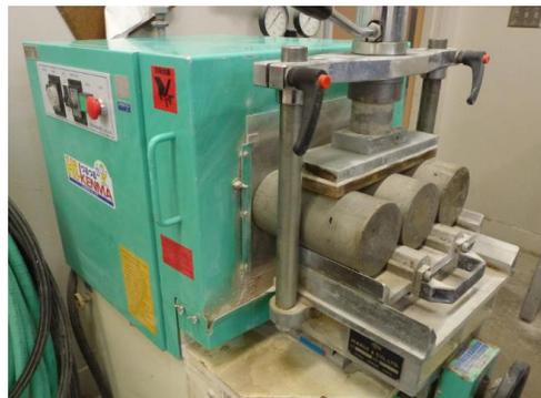
Figure 1. End Grinding Equipment
