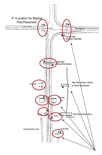
The area around the delineators, object markers and obstacle is to be clear from all tall grass as identified with a red oval if it's in the area that is machine mowed.
