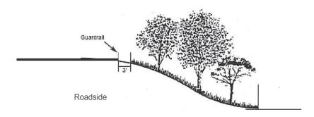
C. Mowing is not required on slopes that are 3:1 or steeper. Mowing section for final snow mowing is to be extended as much as practical towards the toe of the slope as shown in the diagram below. Do not mow up the slope.
