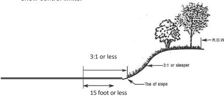
E. Slopes that are flatter than 3:1, either in a cut or fill section shall be mowed as shown in this diagram for snow control.
