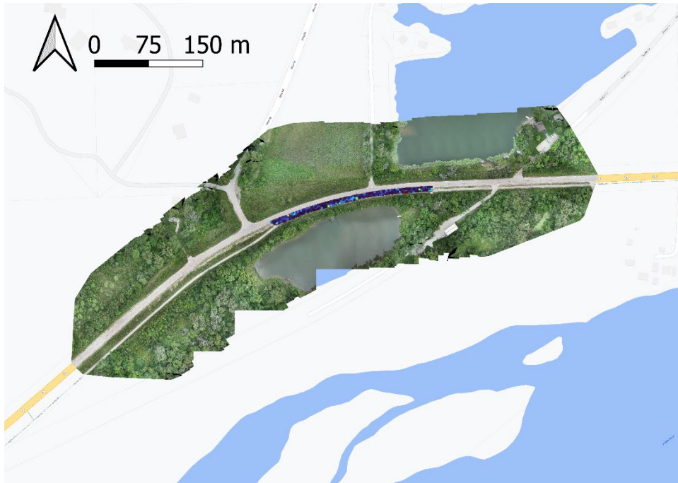
Figure 6.2 Overview of the UAS surveyed area, with the point cloud section used in the analysis shown in predominately blue points
