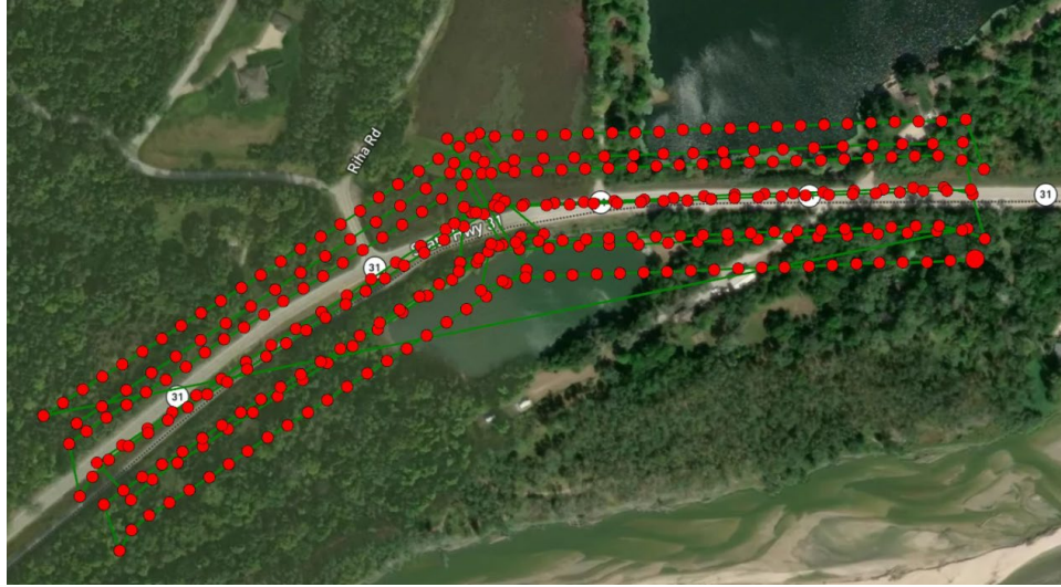
Figure 6.1 UAS survey flight path (with image locations shown in red) for NE-31 near Louisville, Nebraska
