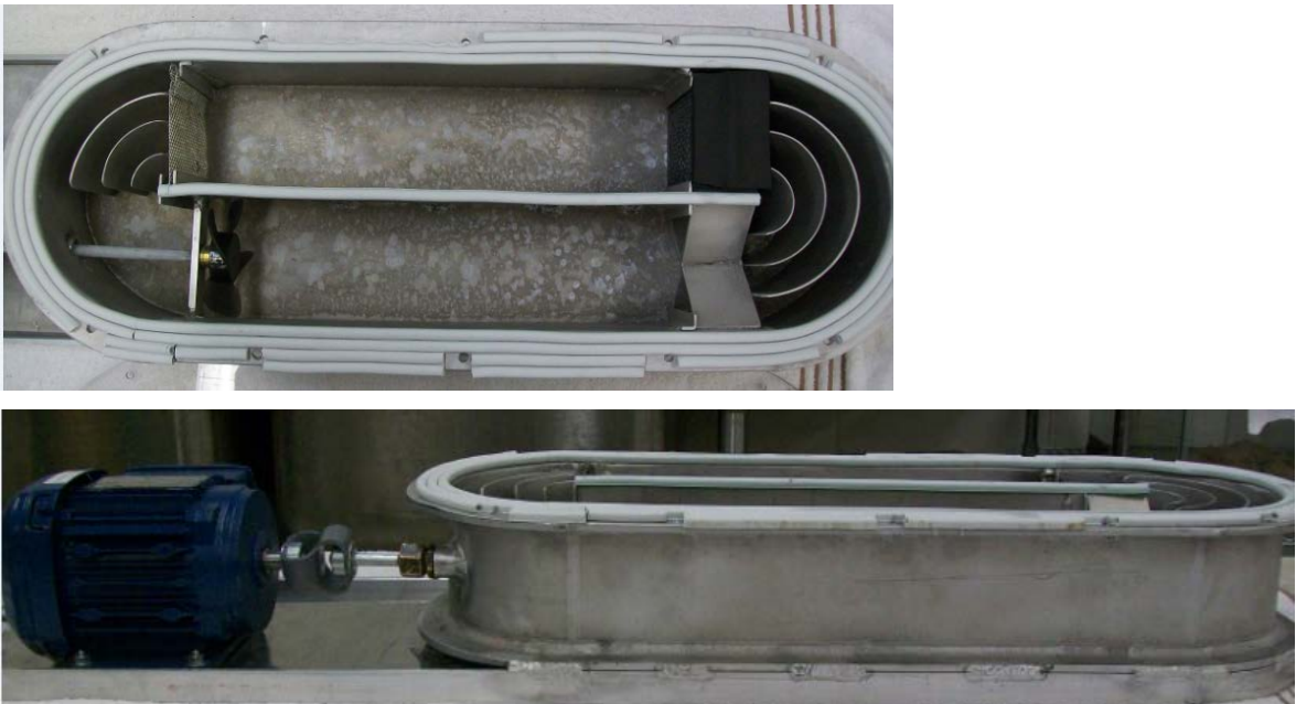
Figure 2-1: Ten liter swim tunnel used to test fish swimming speed
