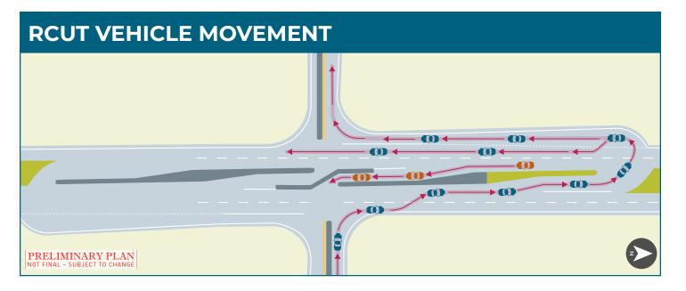
RCUTs have been shown to decrease right-angle crashes on four-lane divided highways. An RCUT intersection requires a change in how drivers cross and turn onto the highway from side roads by preventing direct crossing and left-turn movements. Relative to many other improvements, it is a lowcost treatment that can be guickly implemented, requires minimal property acquisition or relocation of homes and businesses, and minimizes environmental impacts.
