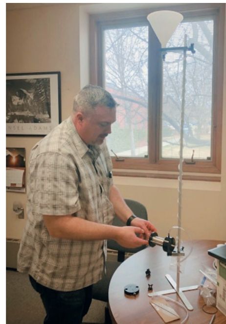
Left - Former Geotechnical Engineer Mark Lindemann demonstrating the pin-hole test.
