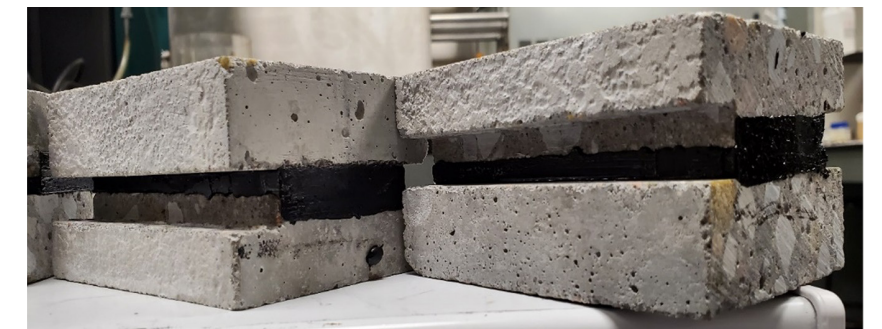
Specially designed concrete blocks allowed Pavement Design to study the bond of hot-pour sealant in narrow saw-cut joints.
