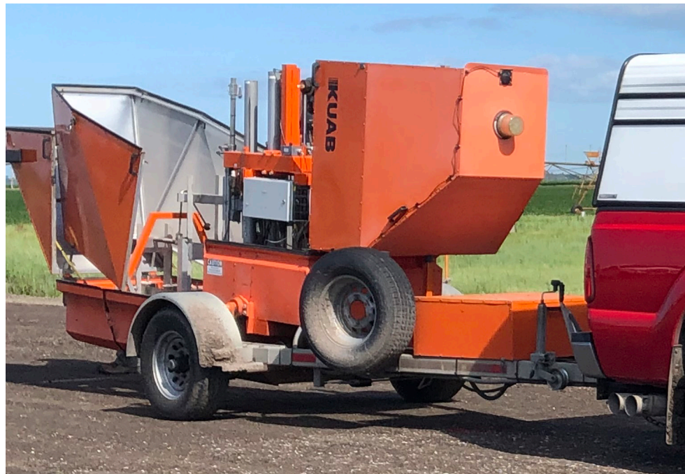
Falling Weight Deflectometer (FWD) measures modulus via deflection with seven sensors and machine-dropped weights.
