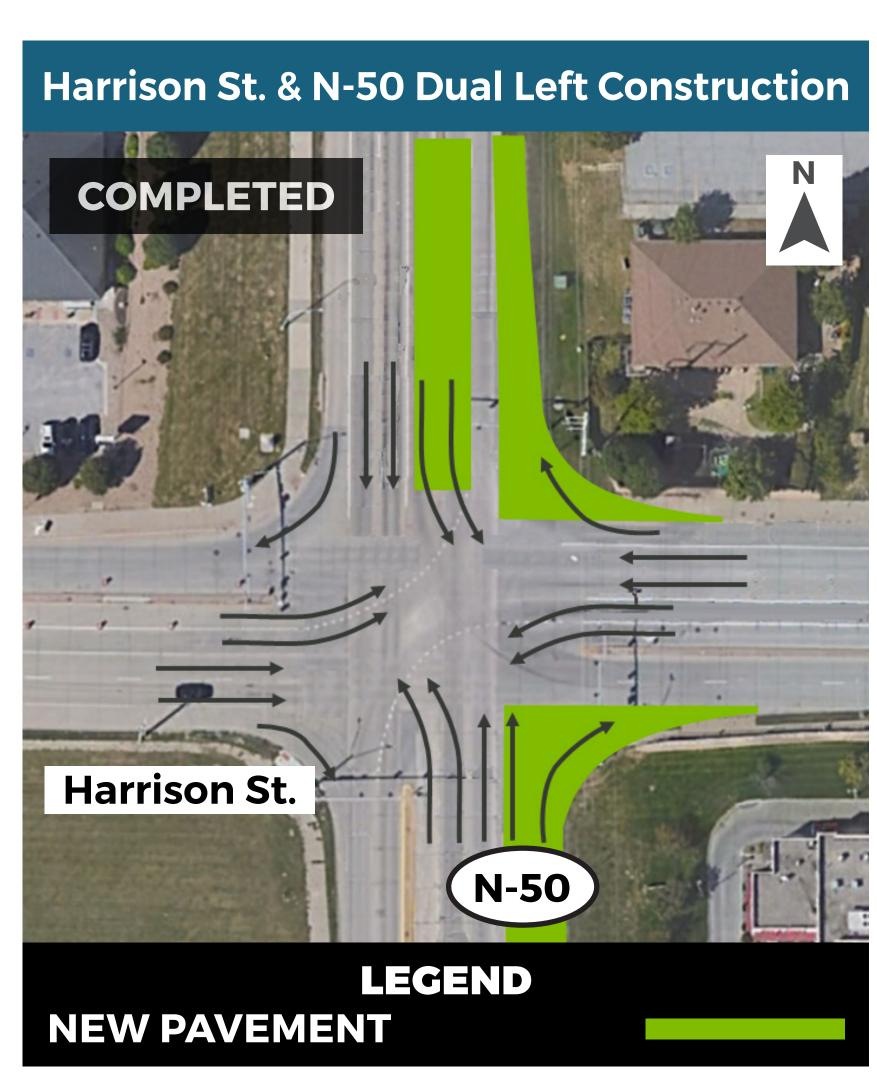
N-50 will be widened along the east side approximately 1,000 feet north & south of the intersection with Harrison Street to include room for two through driving lanes in each direction, two left-turn lanes, and a single right-turn lane.
