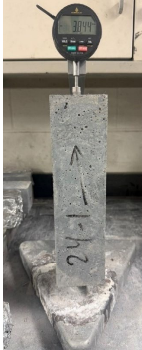
Figure 3.21 Drying shrinkage test setup.
