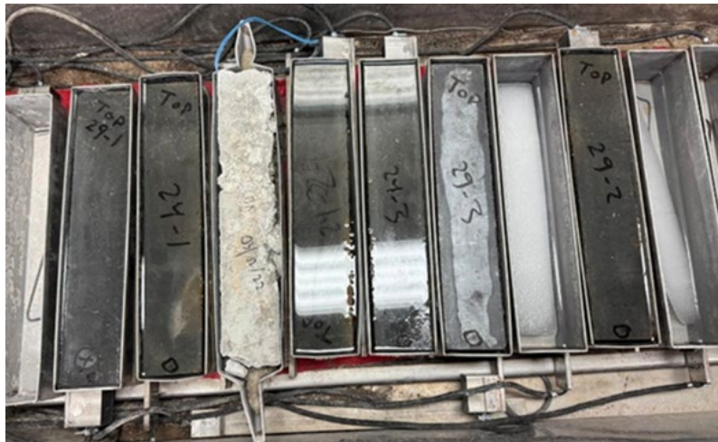
Figure 3.17 UHPC specimens in the freeze-thaw chamber.
