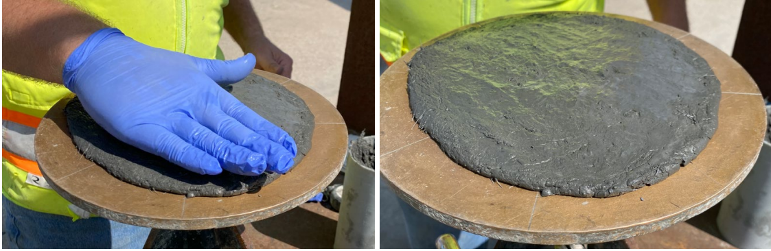
Figure C.6 Material reacts well under external energy (vibration).
