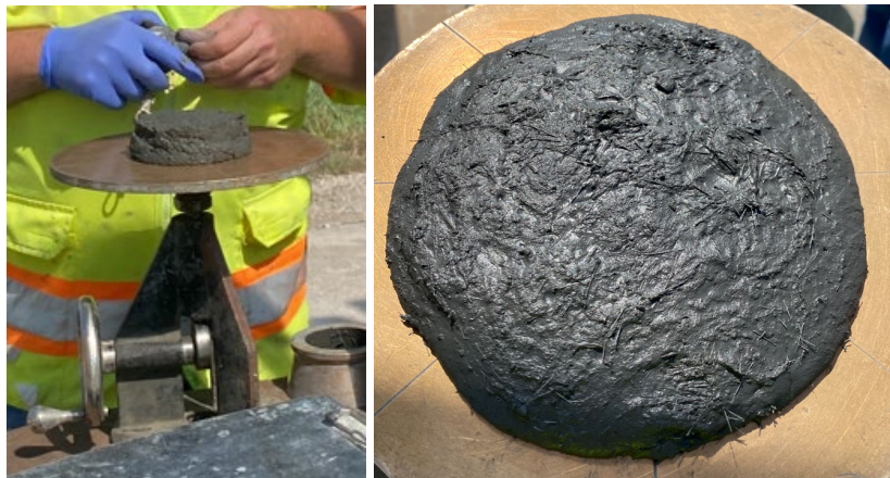
Figure C.5 Flow after adjustment (4.25” static, 7.5” dynamic).
