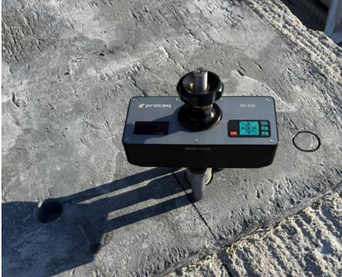
Figure 3.15 Bond strength test setup.
