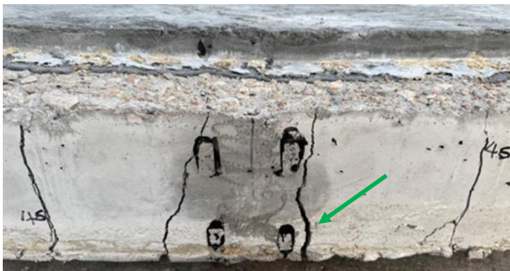
Side view (Cracks in tension side)
