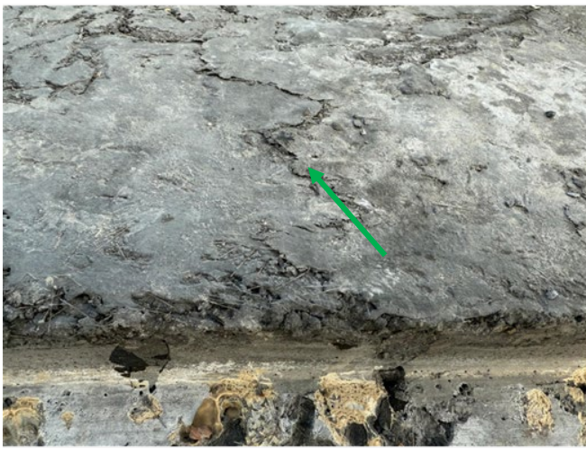
Top view (Crushing of UHPC)
