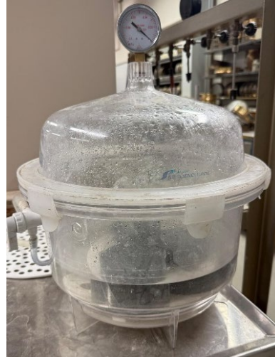
(b) Sample preparation in vacuum saturation chamber
