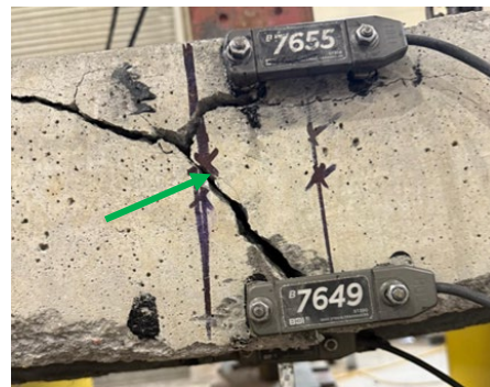
Side view (cracks in tension side and crushing of NC after the rupture of the UHPC layer)
