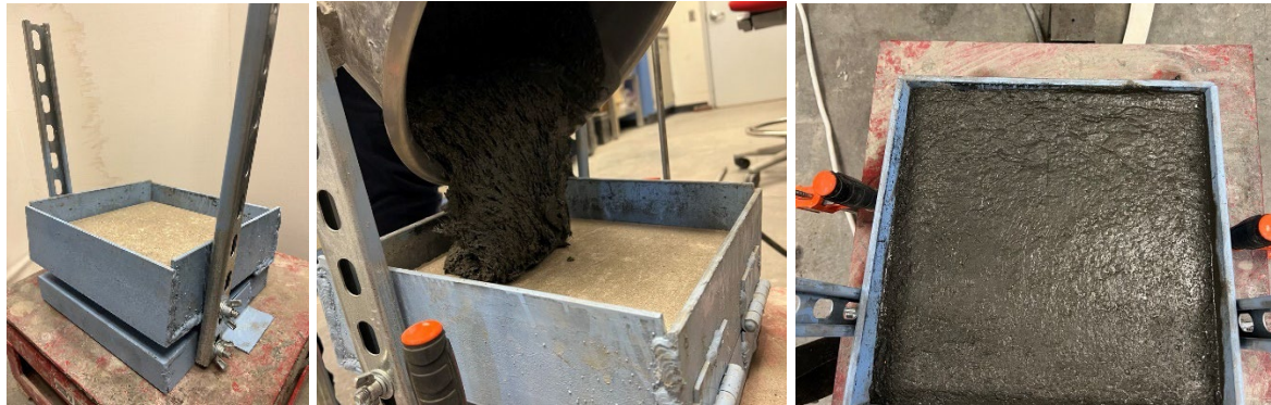
Figure 3.6 Vibration-Slope Stability (VSS) test setup and process.
