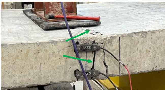
Side view (cracks in tension side and crushing of NC after the rupture of the UHPC layer)
