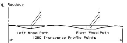
The calculated rutting amount is determined by the average of the left and right wheelpath. If the difference between the LWP and RWP is more than 6 mm, then we use the lower of the two. If the INO data is out of range then use the three point bumper laser system's average rutting.
