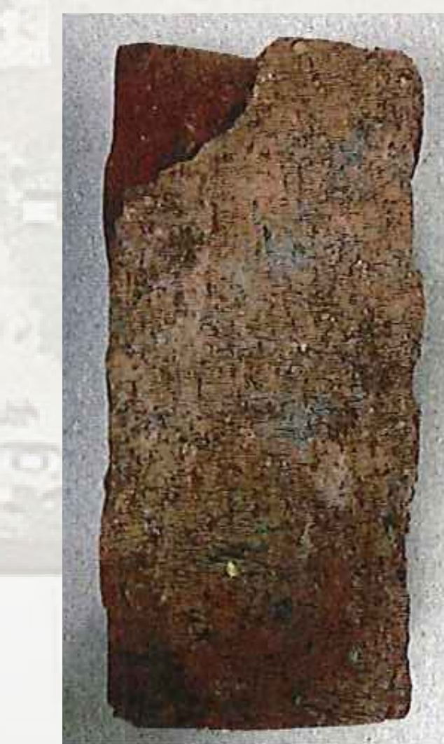
Damage on underside of bricks, not visible from surface
