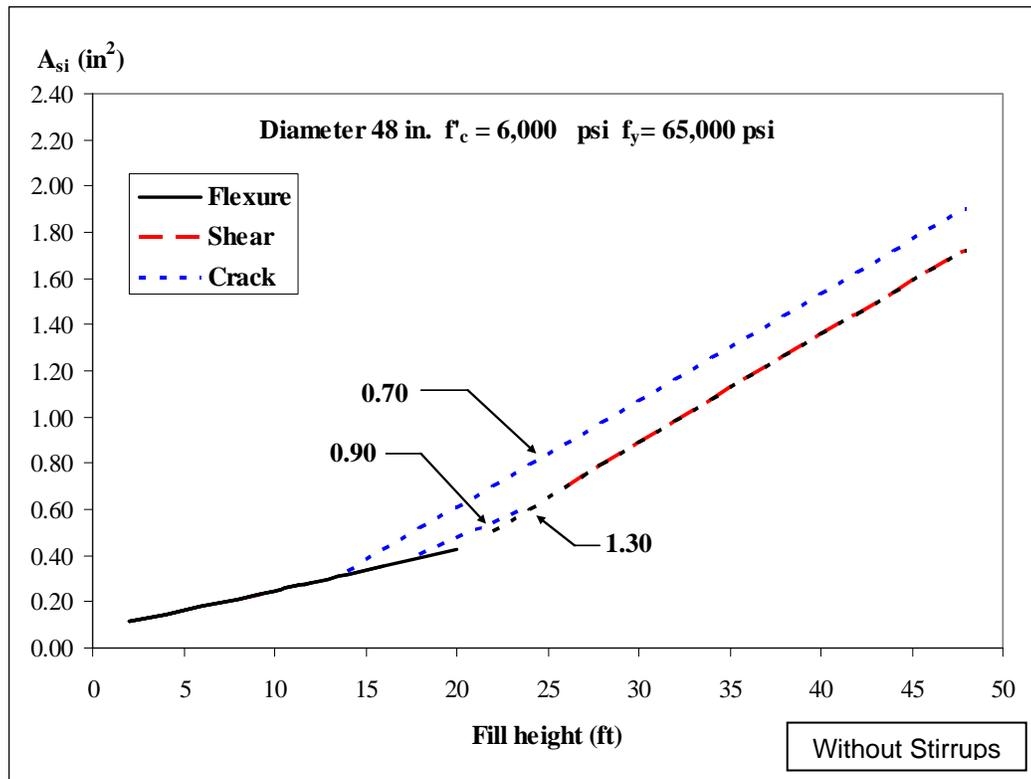
**Figure 7** Parametric Study – Crack Control Factor
