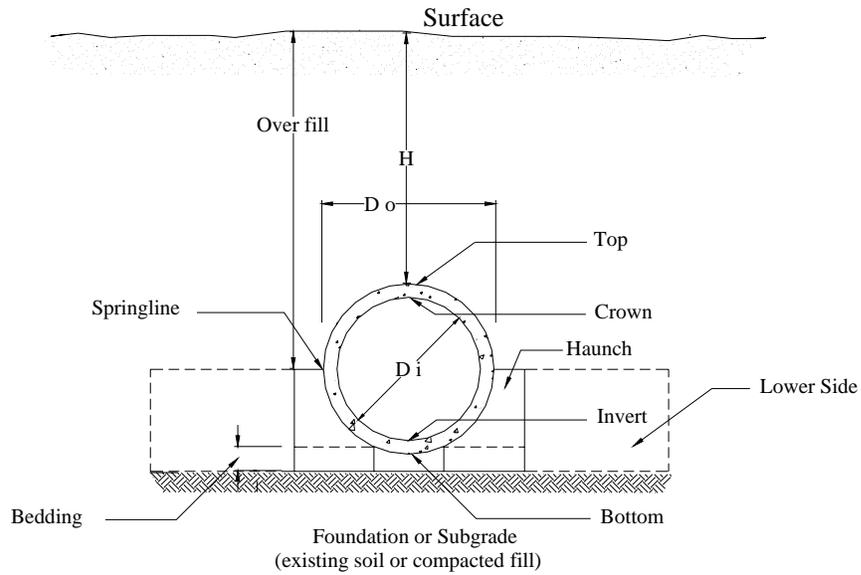
**Figure A-1** Standard Installation Terminology
