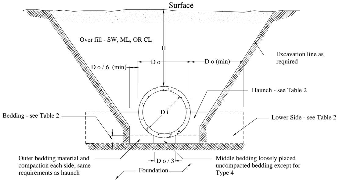
**Figure A-3 Standard Trench Installations**
