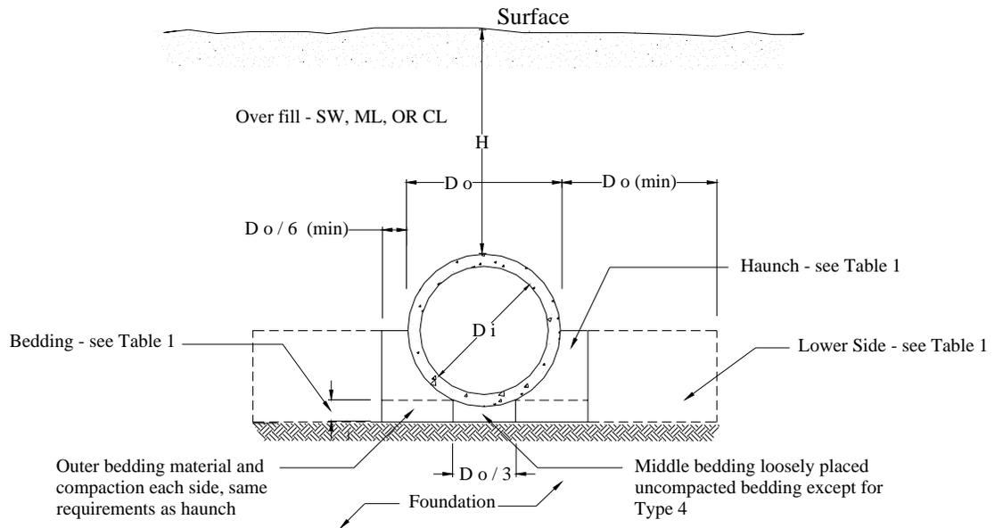
**Figure A-2** Standard Embankment Installations
