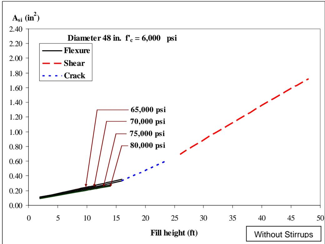
**Figure 5 Parametric Study – Reinforcing Steel Strength**
