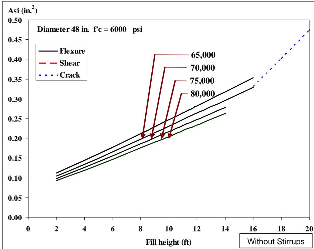
**Figure 6** Parametric Study – Reinforcing Steel Strength
