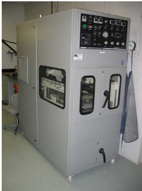
**Figure 3.6** APA Testing Machine
