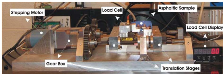
**Figure 3.11** Fracture-Damage Testing Device Set-up (Freitas *et al.* 2006)
