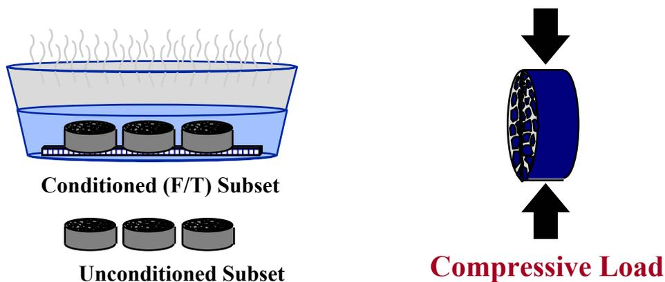
**Figure 3.4** Schematic View of AASHTO T-283 Testing
