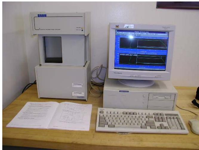
**Figure 3.14** Wilhelmy Plate Testing Device
