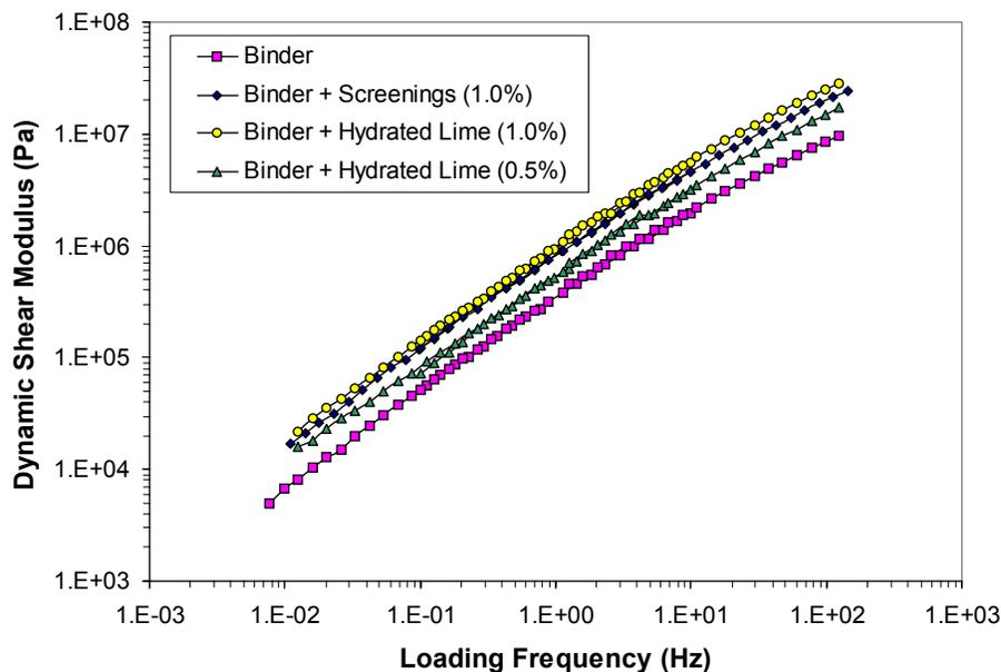
**Figure 4.12** Master Curves at 30°C of Each Binder/Mastic
