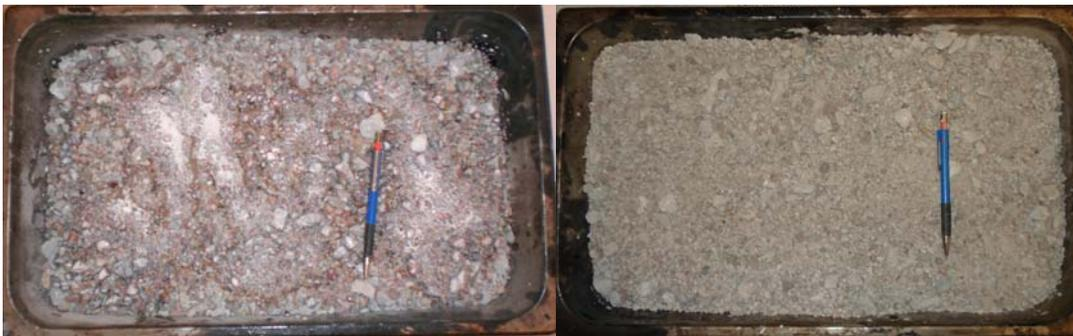
**Figure 4.10** Diluted Lime Slurry Treated Aggregates (Before and After Oven Dry)
