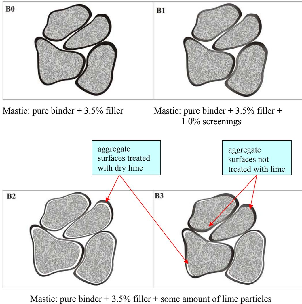
**Figure 4.11** Illustrations Representing Mastic-Aggregate System of Each Mix
