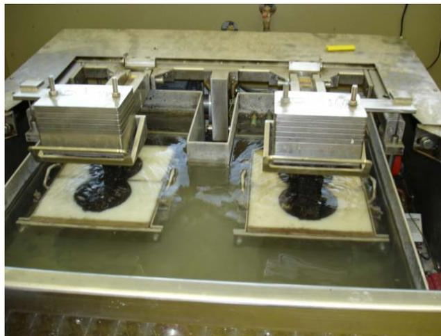
**Figure 4.6** Hamburg Specimens under Testing
