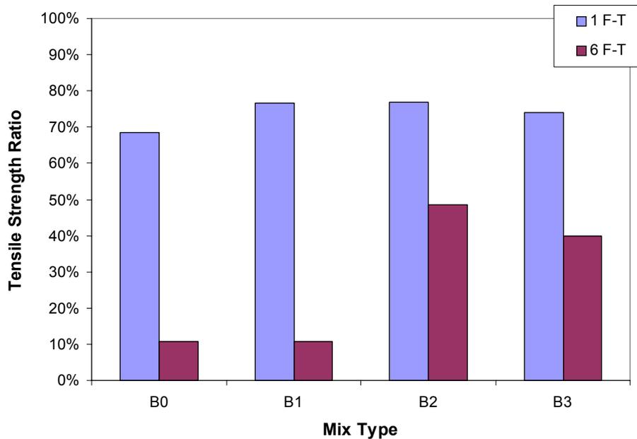
**Figure 4.2** Tensile Strength Ratio of Each Mix
