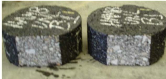
**Figure 4.5** Hamburg Specimens After Being Cut
