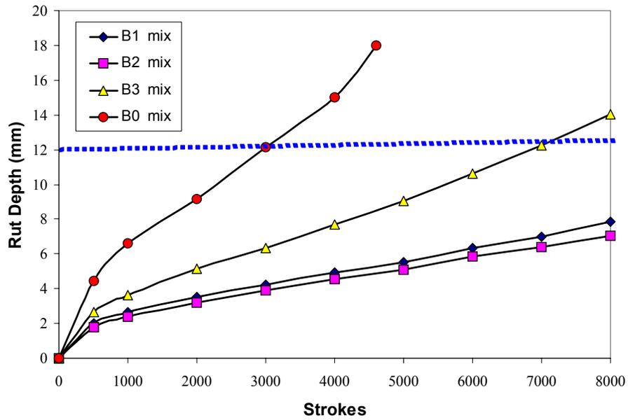
Figure 4.3 Continuous APA Rut Depths of Each Mix
