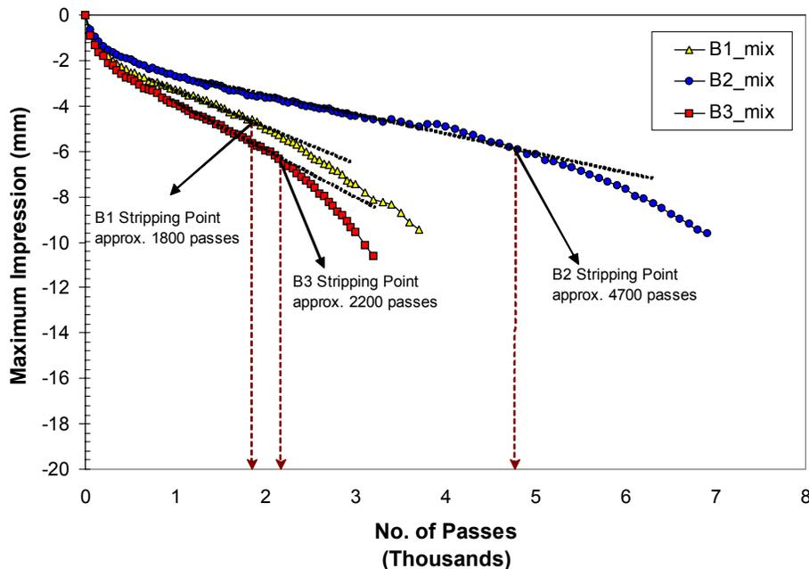
**Figure 4.7** Hamburg Testing Results of Each Mix
