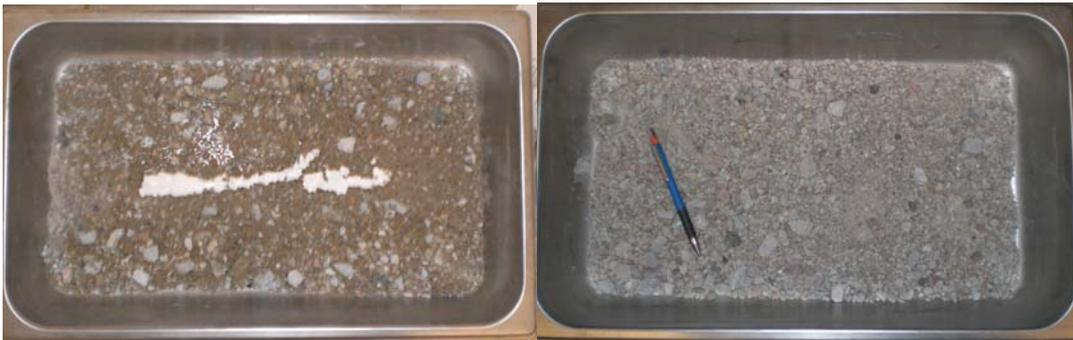
**Figure 4.9** Lime Slurry Treated Aggregates (Before and After Oven Dry)
