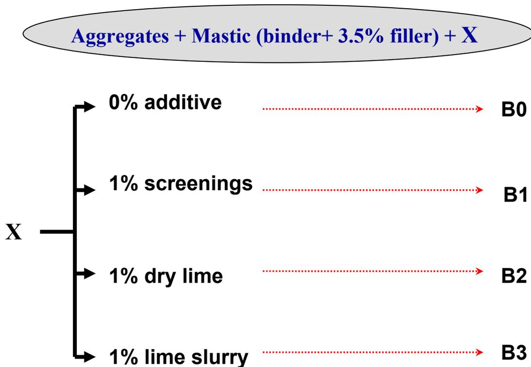
Figure 3.1 SP2 Mixes Designed (B0, B1, B2 and B3)
