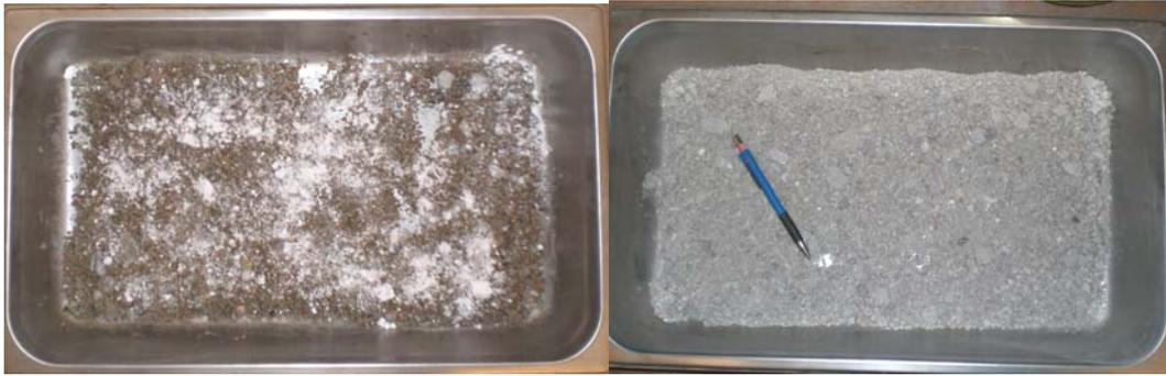
**Figure 4.8** Dry Lime Treated Aggregates (Before and After Oven Dry)
