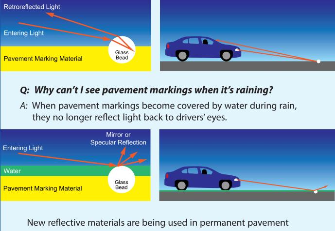
New reflective materials are being used in permanent pavement markings on many different roadways. These materials are more visible during wet conditions. Unfortunately, during heavy rains the pavement markings may become flooded and, therefore, less visible.
